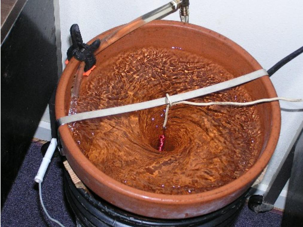
Swirler in inflow mode (CCW) showing placement of the grounding coil.
