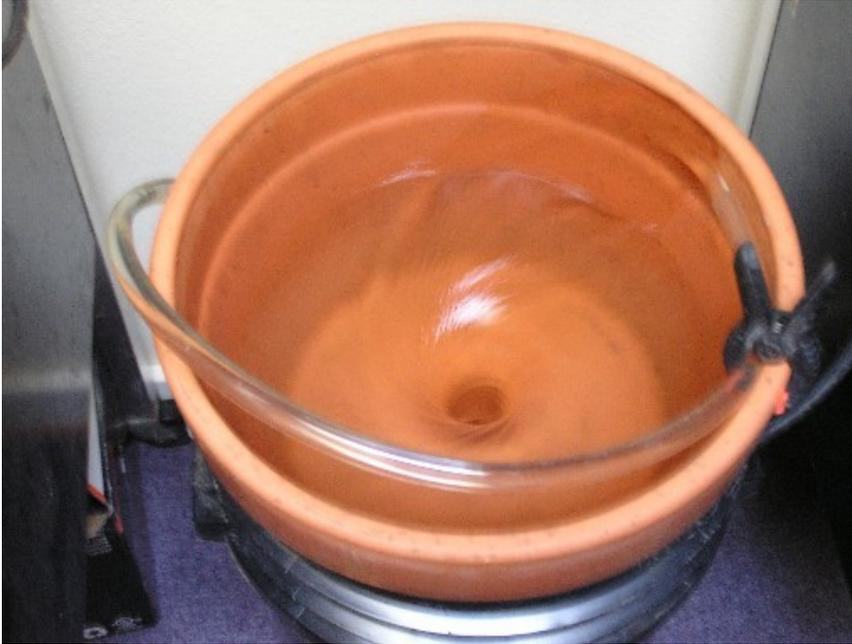
A simple swirler setup utilizing a clay flowerpot setting into a 5 gallon bucket, and showing a counter-clockwise vortex. Wooden wedges were added to this setup to create a gap, which allows the hose and pump cord to pass into the sump. A 90 degree brass elbow was later added to reduce the hose length required and make it more aesthetically looking. It also makes it easier to switch between ccw and cw vortex flow.
