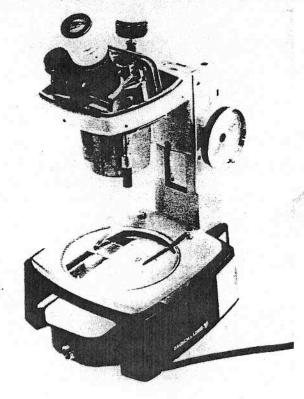
Loosen two screws that hold the E.F. Assembly and cement if needed. By moving the E.F. Assembly you can straighten the zoom. Then adjust the mirror to bring the image to within ½mm of center.
