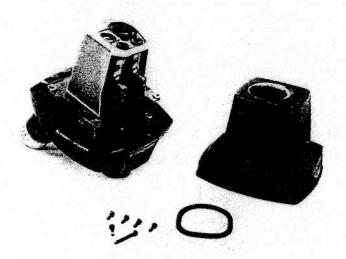
Remove the Objective Cover and Cover Gasket. The Objective Cover is attached with six screws.
