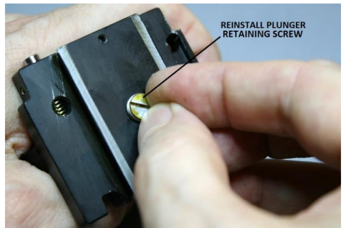
Figure 39 – Reinstall the plunger-retaining screw
