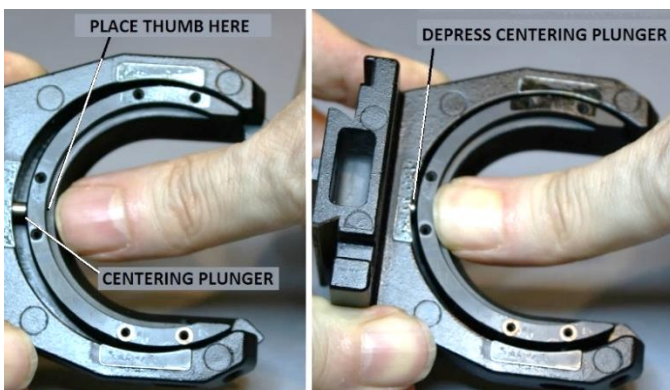
Figure 12 – Depress the centering plunger
