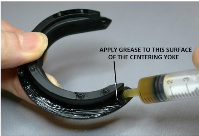
Figure 46 – Lightly grease the underside of centering yoke
