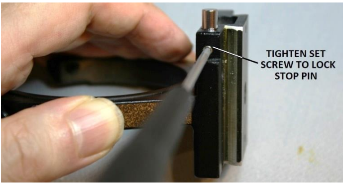
Figure 28 – Tighten set screw to lock the stop pin
