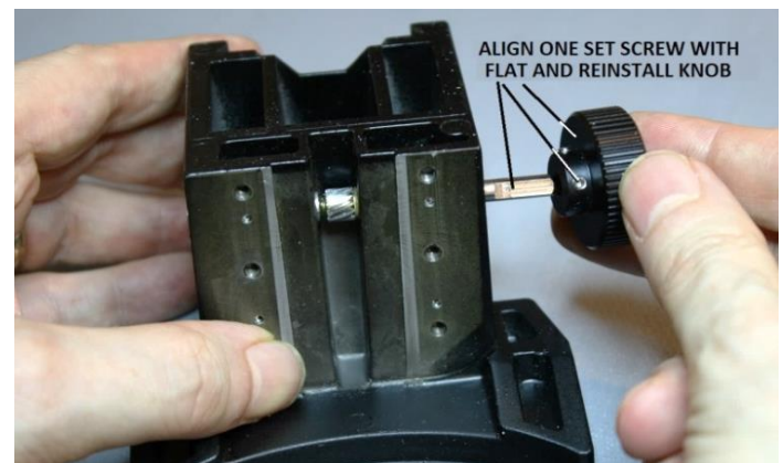
Figure 93 – Reinstall knob onto condenser-height shaft
