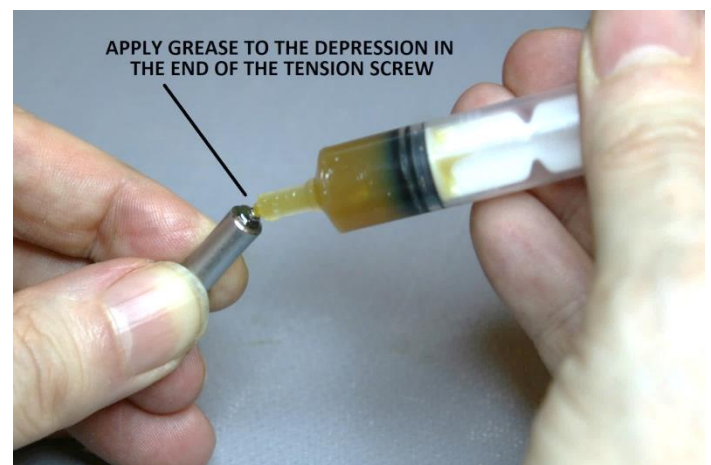
Figure 87 – Apply grease to the end of the tension screw
