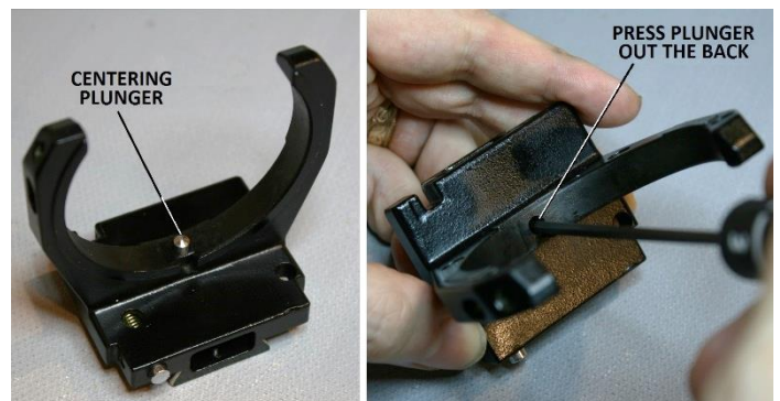
Figure 33 – Press centering plunger out the back of bore
