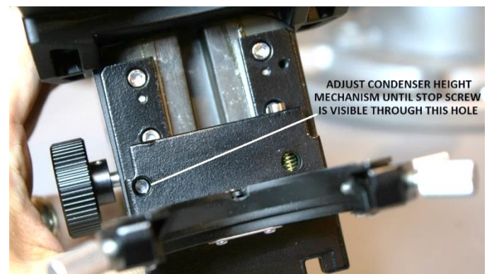
Figure 2 – Adjust condenser height until screw is visible
