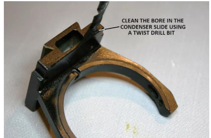
Figure 25 – Clean any debris or burring from the bore
