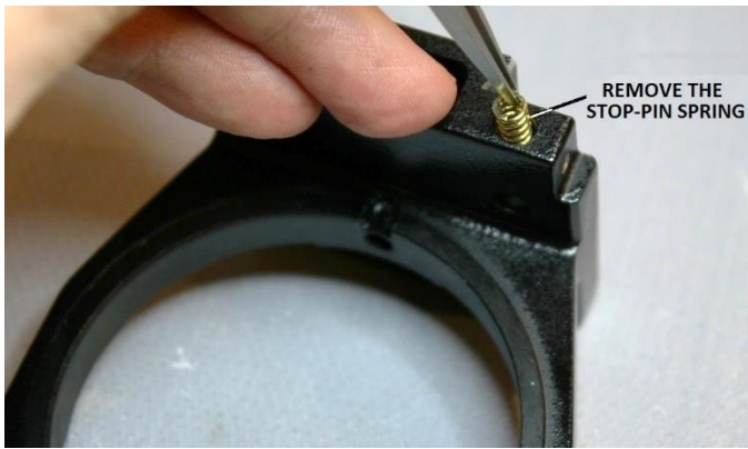
Figure 22 – Remove the stop-pin spring from the slide
