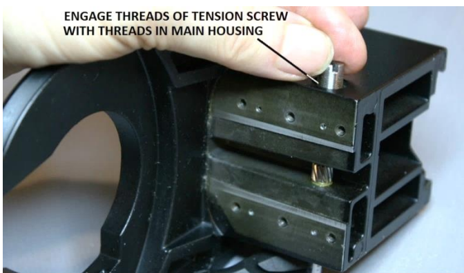
Figure 90 – Engage threads of tension screw with housing
