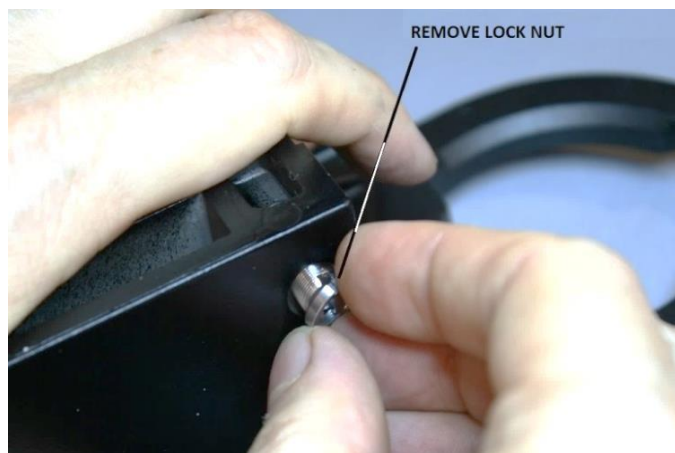
Figure 69 – Unscrew and remove tension-screw lock nut
