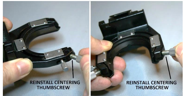
Figure 55 – Reinstall the centering thumbscrews
