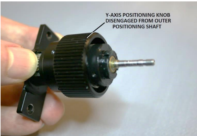
Figure 16 – Y-axis knob disengaged from the outer shaft
