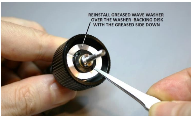
Figure 52 – Reinstall wave washer onto the backing disk
