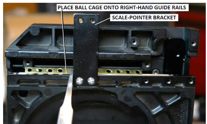
Figure 127 – Place ball cage onto right-hand guide rails
