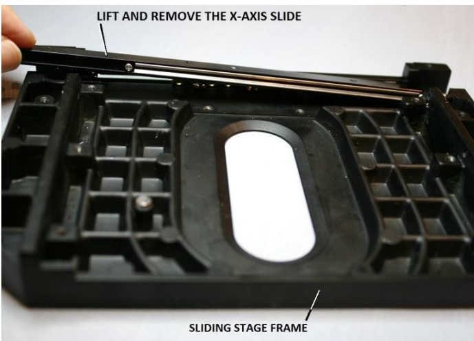
Figure 101 – Lift and remove the X-axis slide
