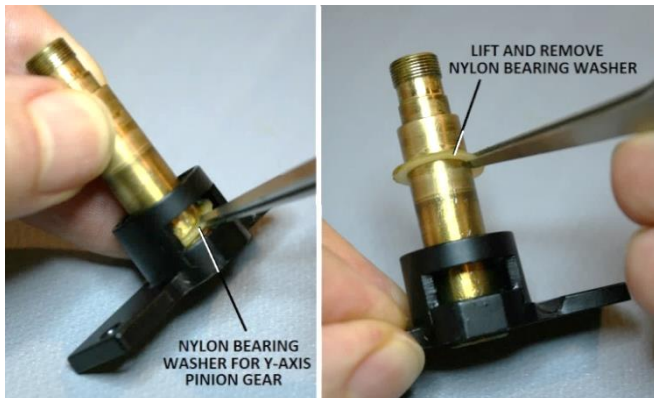
Figure 28 – Carefully remove the large nylon washer
