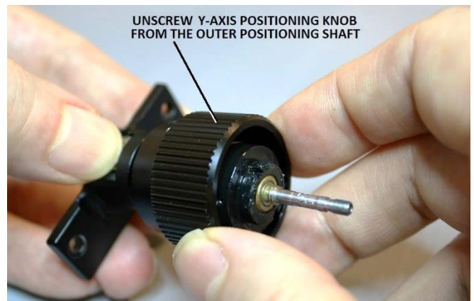
Figure 15 – Unscrew the Y-axis knob from the outer shaft
