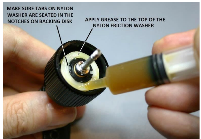
Figure 55 – Apply grease to the top of the nylon washer
