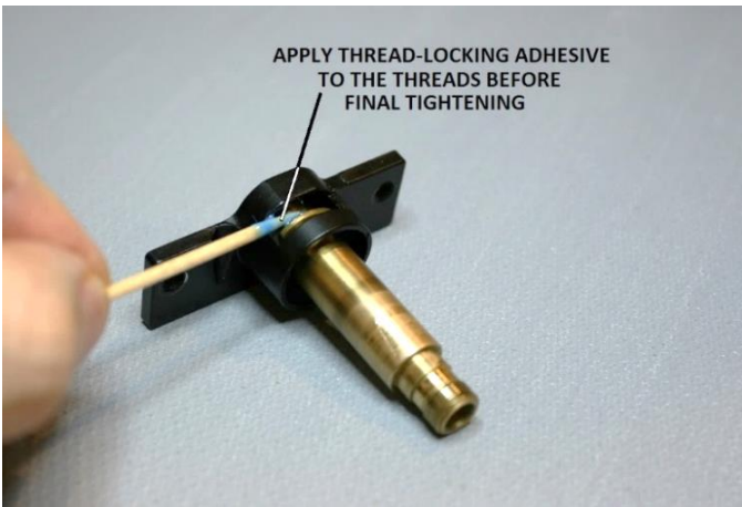
Figure 33 – Apply Loctite® to threads before tightening
