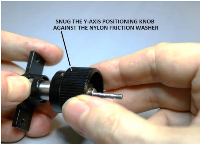
Figure 50 – Snug Y-axis knob against the nylon washer
