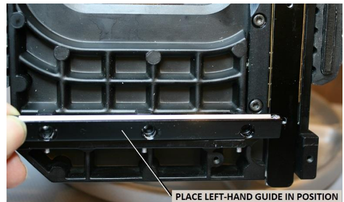
Figure 121 – Place the left-hand guide in position
