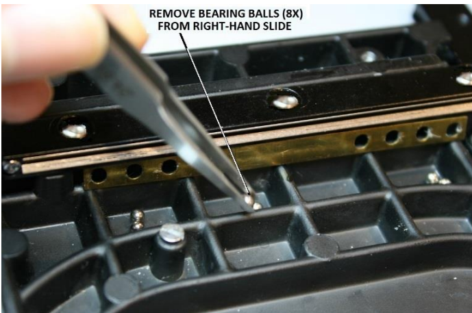
Figure 90 – Remove bearing balls from right-hand slide
