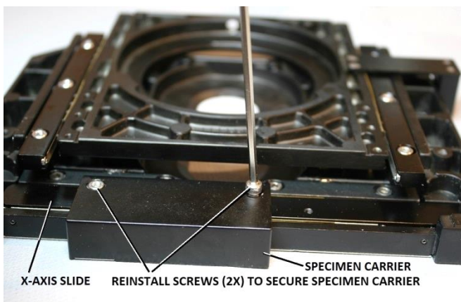
Figure 136 – Secure the specimen carrier in position
