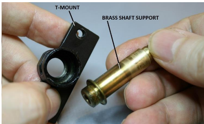
Figure 30 – Separate brass shaft support from T-mount
