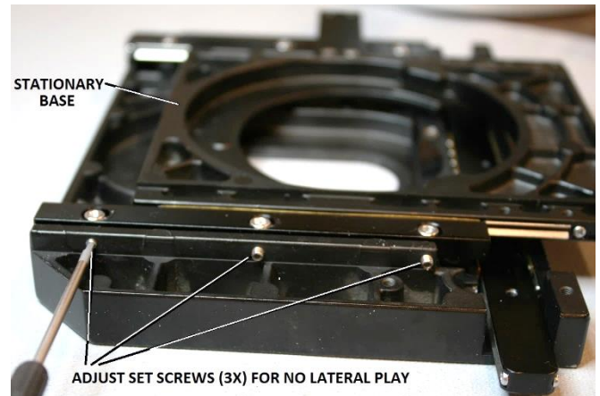
Figure 132 – Adjust set screws for no lateral play
