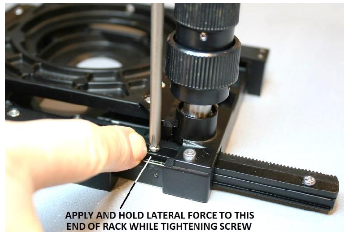
Figure 144 – Adjust left-most end of the X-axis rack
