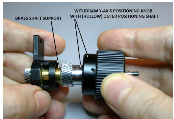
Figure 21 – Withdraw the Y-axis knob and the outer shaft
