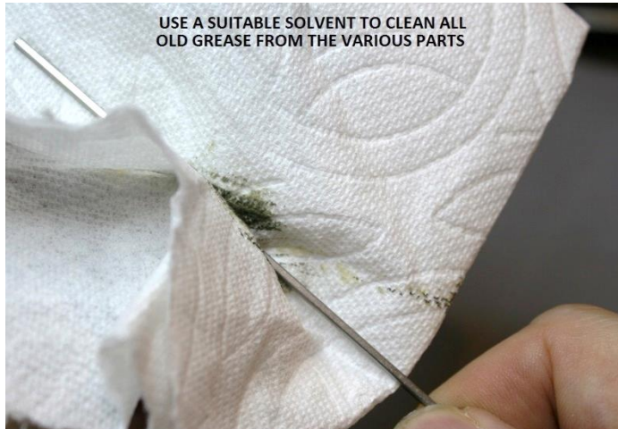
Figure 160 – Remove all old grease from the parts
