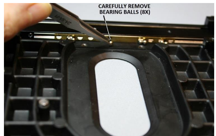
Figure 99 – Remove bearing balls from the front of slide
