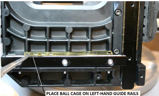
Figure 123 – Place ball cage on the left-hand guide rails
