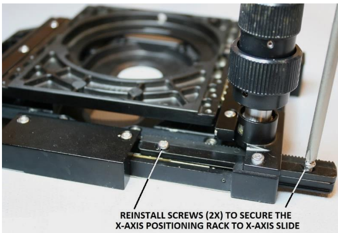
Figure 142 – Reinstall X-axis positioning rack screws
