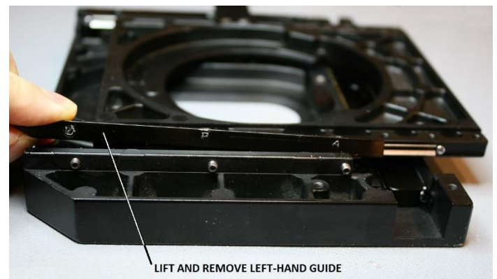
Figure 86 – Lift and remove the left-hand guide
