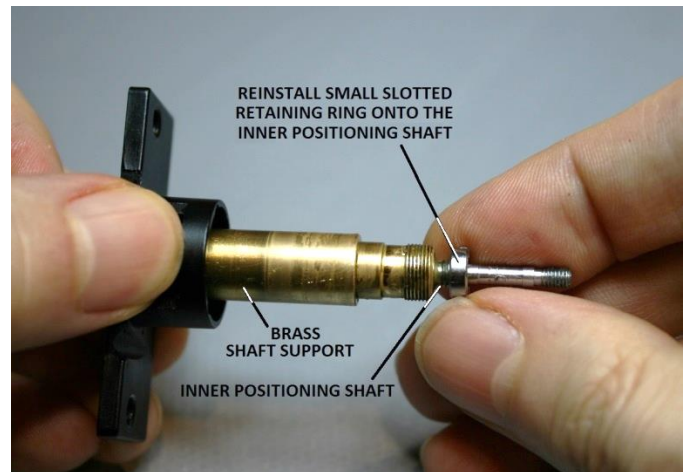
Figure 37 – Reinstall the slotted retaining ring
