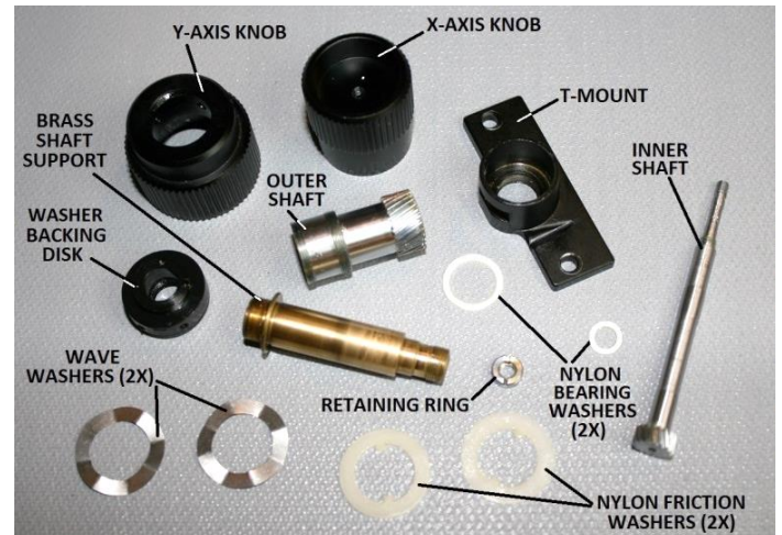
Figure 31 – Components of coaxial positioning assembly
