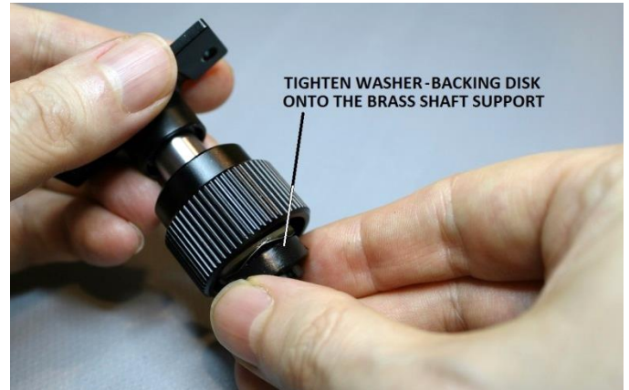
Figure 48 – Screw backing disk onto brass shaft support
