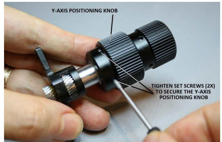
Figure 58 – Tighten set screws for the Y-axis knob
