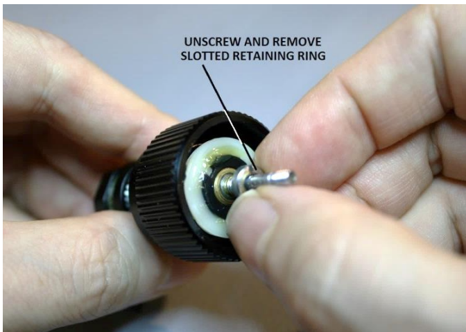
Figure 11 – Unscrew and remove slotted retaining ring
