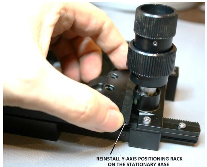
Figure 147 – Hold the Y-axis positioning rack in place
