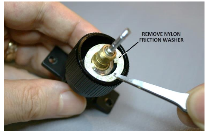
Figure 20 – Remove nylon washer under wave washer
