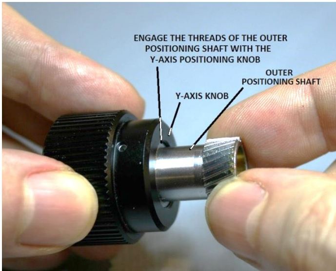
Figure 39 – Engage the threads of outer shaft with knob
