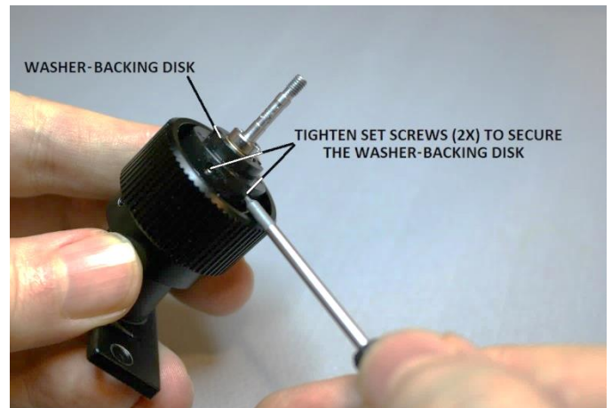
Figure 49 – Tighten the set screws on the backing disk
