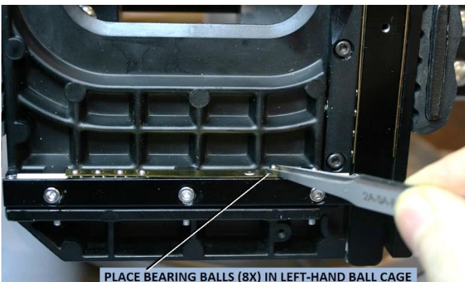
Figure 124 – Place bearing balls in the left-hand ball cage
