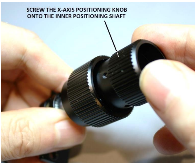
Figure 56 – Screw the X-axis knob onto the inner shaft
