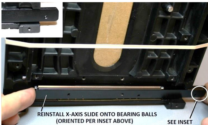
Figure 113 – Place X-axis slide onto the rear bearing balls
