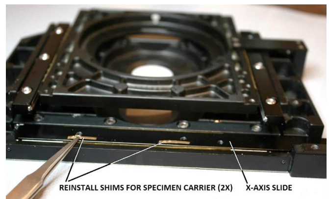
Figure 134 – Reinstall any shims for the specimen carrier
