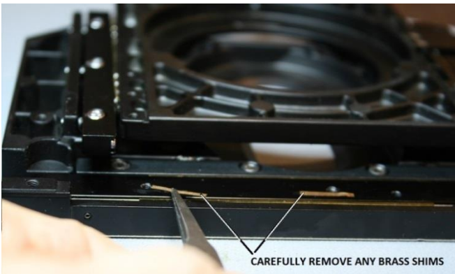
Figure 82 – Remove brass shims (if preset) from slide
