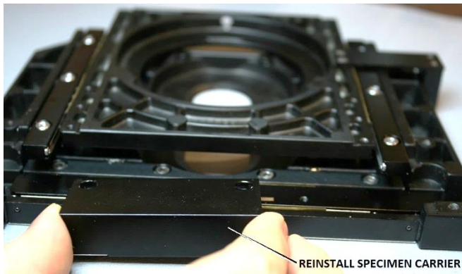
Figure 135 – Place the specimen carrier in position
