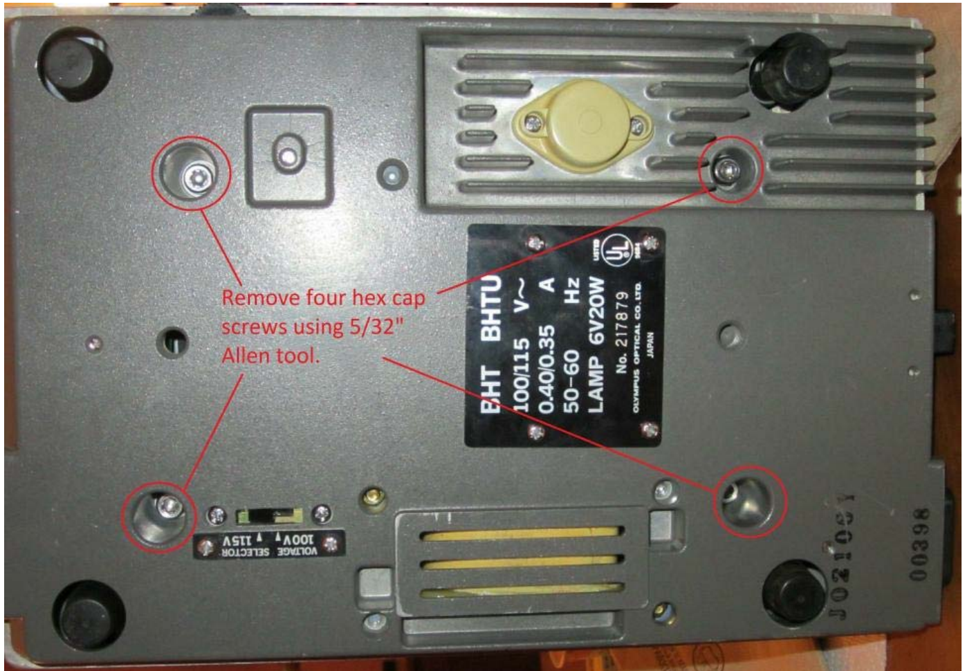
Figure 4 – Bottom View of BHT/BHTU Electrical Base (100/115V Version)
