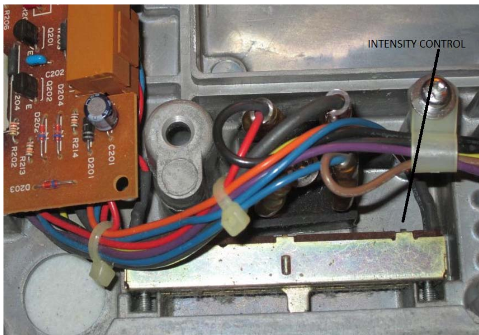
Figure 9 – Lamp Intensity Control Mounted to BHT/BHTU Electrical Base (100/115V Version)
