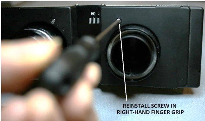
Figure 128 – Reinstall front screw into the finger grip (right)
