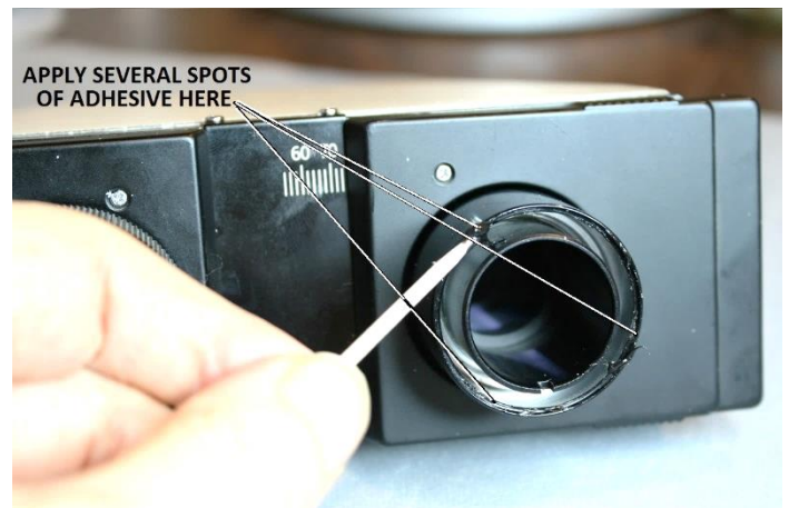
Figure 135 – Apply spots of adhesive to ocular tube (right)
