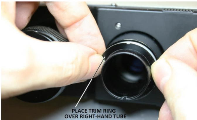
Figure 136 – Place trim ring over the ocular tube (right)
