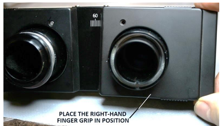
Figure 127 – Place the finger grip into position (right)
