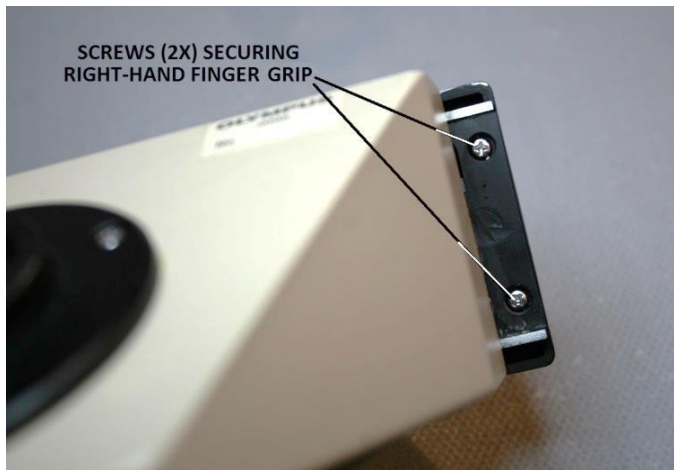
Figure 9 – Screws securing finger grip to slide (right)
