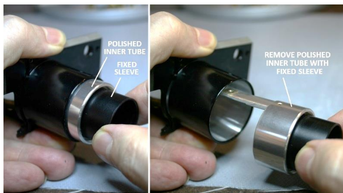
Figure 76 – Remove sleeve/inner tube from ocular tube (right)
