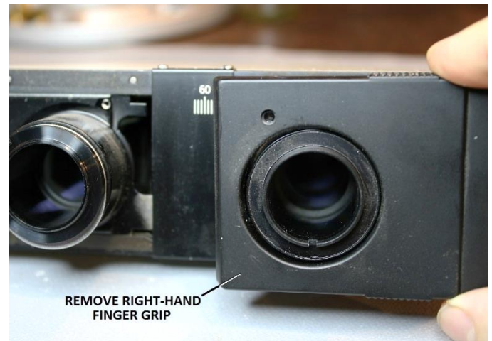
Figure 12 – Remove finger grip from ocular tube (right)
