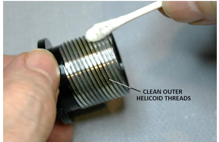
Figure 36 – Clean old grease from the outer helicoid threads
