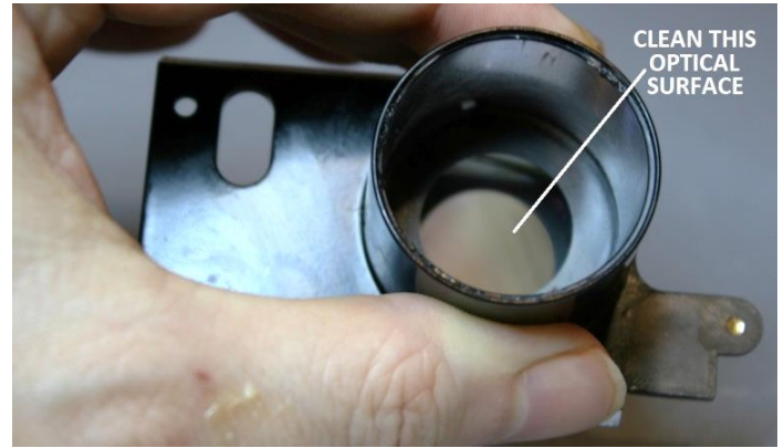
Figure 83 – Clean face 2 of the P6 prism (left)
