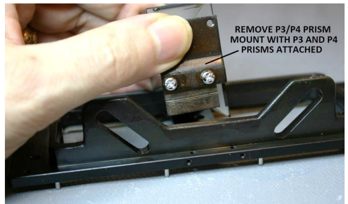
Figure 68 – Remove P3/P4 prism mount with prisms
