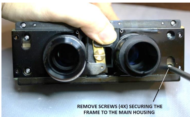
Figure 17 – Remove screws securing front frame to housing
