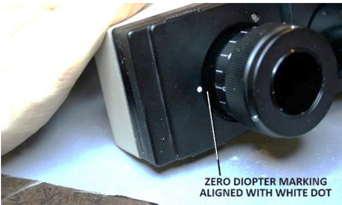
Figure 133 – Align the zero-diopter marking with white dot
