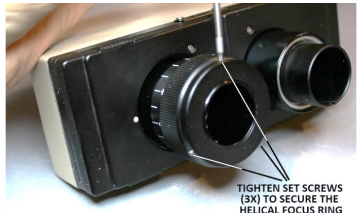
Figure 131 – Tighten set screws to secure helical focus ring
