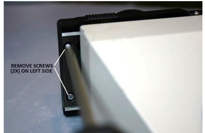
Figure 6 – Remove screws securing finger grip (left)
