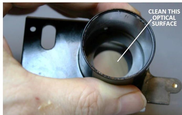
Figure 78 – Clean face 2 of the P5 prism (right)
