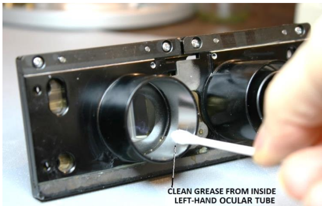
Figure 41 – Remove grease from the ocular tube (left)
