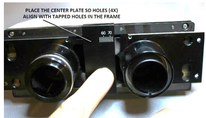
Figure 120 – Position center plate to align with holes in frame
