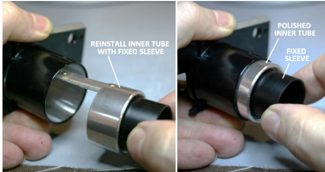
Figure 80 – Reinstall inner tube/sleeve into ocular tube (right)
