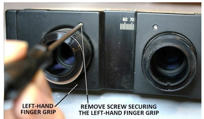
Figure 7 – Remove front screw from finger grip (left)
