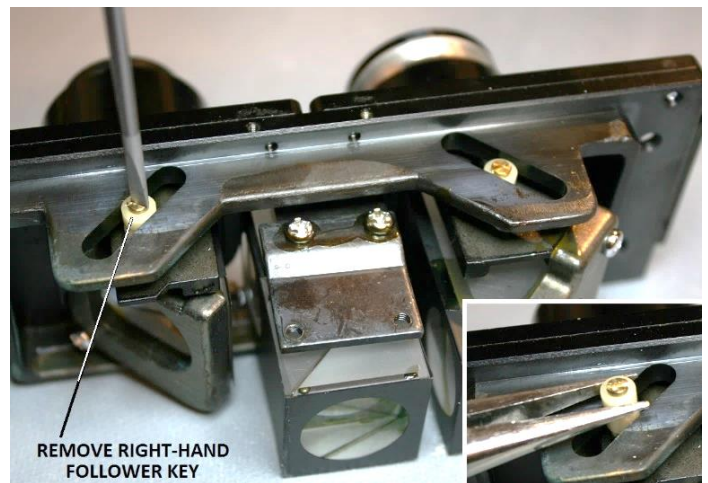
Figure 31 – Remove the follower key (right)
