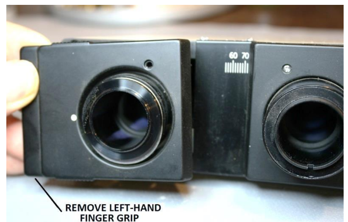
Figure 8 – Remove finger grip from ocular tube (left)
