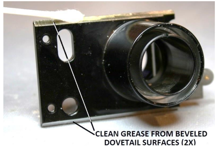
Figure 62 – Clean old grease from bevels of slide (right)
