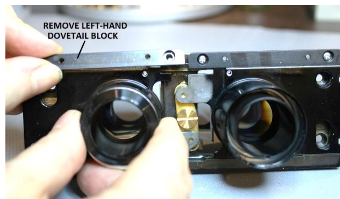
Figure 49 – Remove dovetail block from the frame (left)
