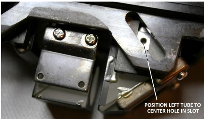
Figure 105 – Position ocular slide to center hole in slot (left)
