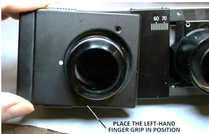
Figure 124 – Place the finger grip into position (left)
