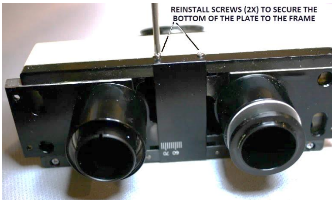
Figure 122 – Secure the plate with two screws (bottom)
