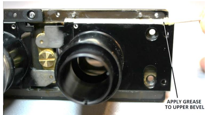
Figure 101 – Apply grease to the upper bevel (right)
