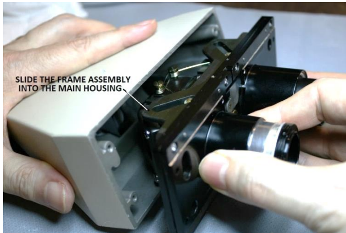
Figure 116 – Slide the frame assembly into the main housing
