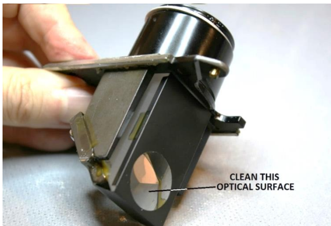
Figure 82 – Clean face 1 of the P6 prism (left)
