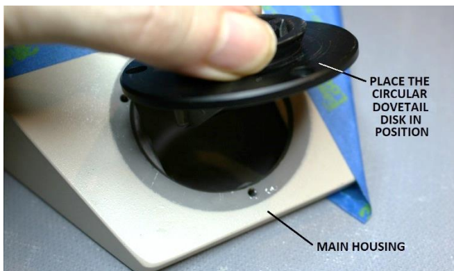
Figure 23 – Place the mounting disk assembly into position
