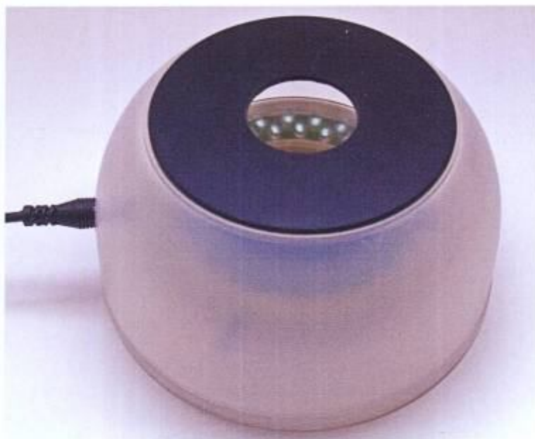
FIG. 2. LED ringlight darkground illuminator.
