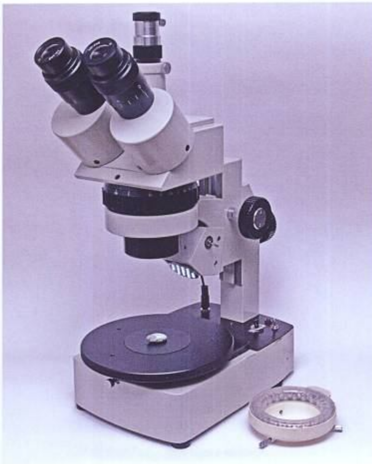
FIG. 5. A stereo microscope fully equipped with LED illumination.
