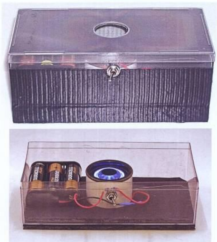
FIG. 3. Watson "Spot-Lens" small portable darkground illuminator.
