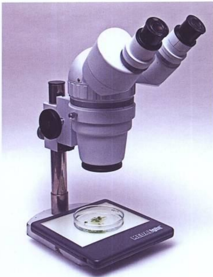
FIG. 1. A basic stereo stand used with a transmitted light panel.
