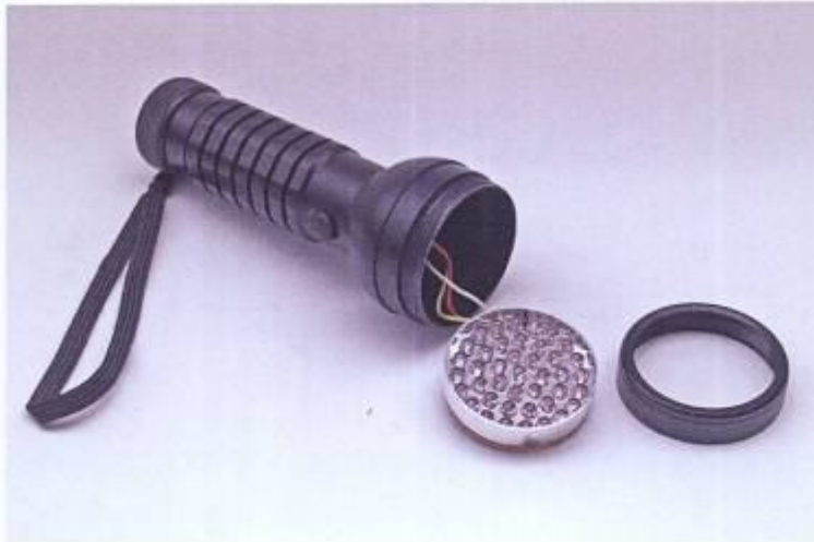
FIG. 4. A torch, disassembled to show the LED array and reflector.
