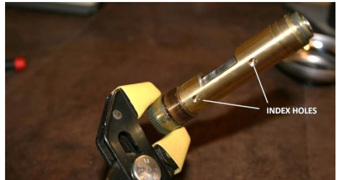
Figure 72 – A view of the index holes in the pinion mount
