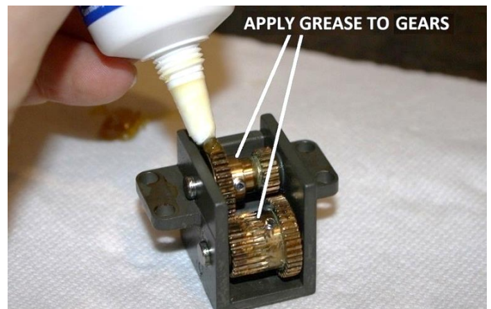
Figure 108 – Apply grease to the teeth of both gears
