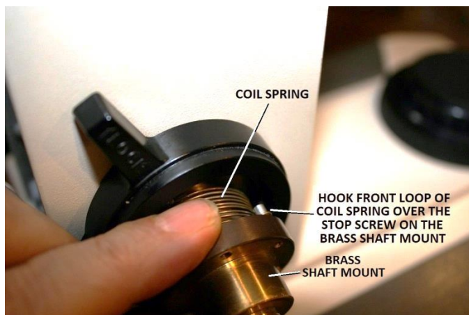
Figure 84 – Place the front loop of spring over stop screw
