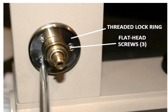
Figure 78 – Reinstall the threaded lock ring
