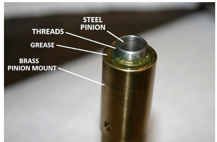
Figure 64 – Apply ring of grease to the retaining ring end
