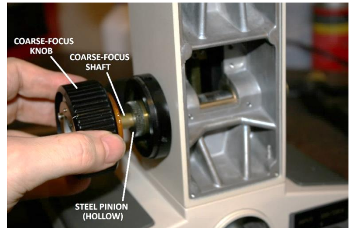
Figure 77 – Slide coarse-focus shaft into the hollow pinion
