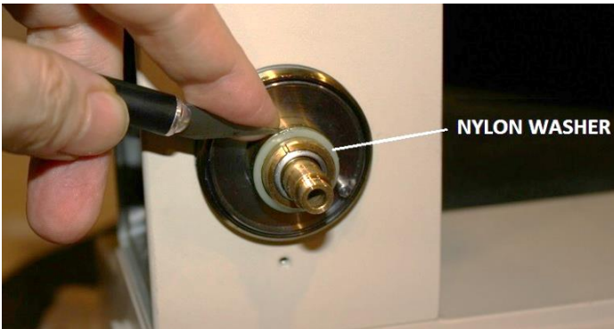
Figure 28 – Remove the nylon washer with X-Acto® knife
