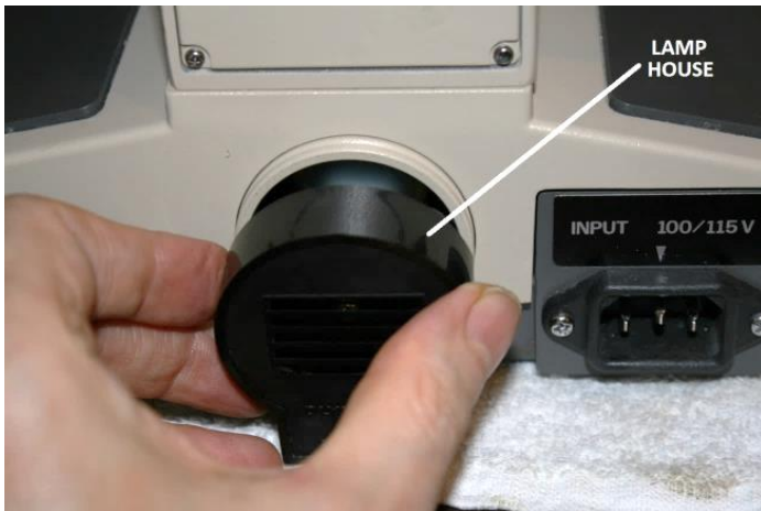
Figure 118 – Reinstall the lamp house on rear of the base
