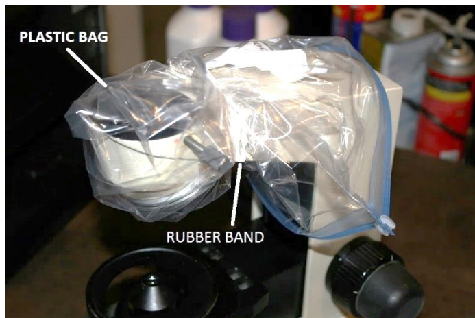
Figure 1 – Protect the top of the arm from dust
