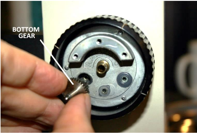
Figure 38 – Remove the bottom (left-most) gear
