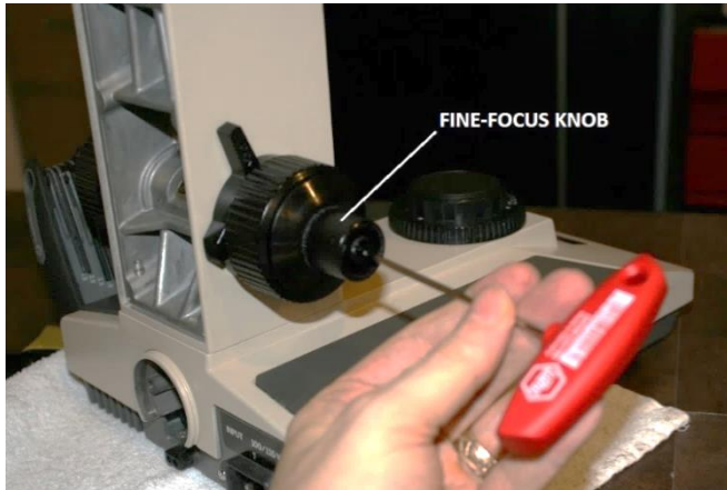
Figure 92 – Reinstall the set screw to secure the knob
