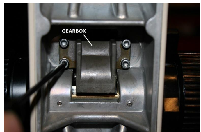
Figure 7 – Remove screws and washers holding gearbox
