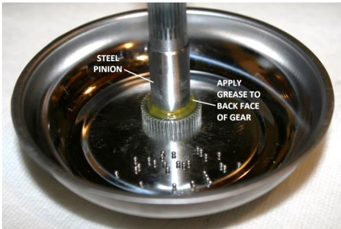
Figure 61 – Apply grease to back face of the pinion gear
