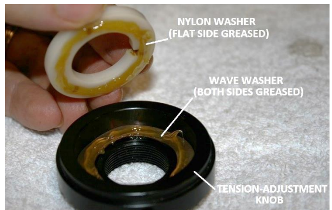
Figure 68 – Reinstall the greased nylon tension washer
