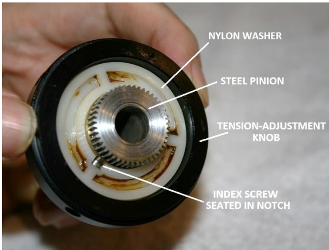
Figure 70 – Snug the tension-adjustment knob
