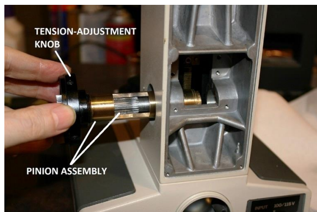
Figure 51 – Withdraw the pinion assembly from frame
