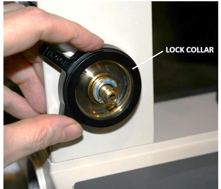
Figure 81 – Reinstall the pre-focus lock collar
