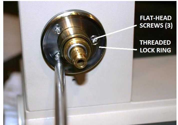
Figure 30 – Remove screws holding the threaded lock ring
