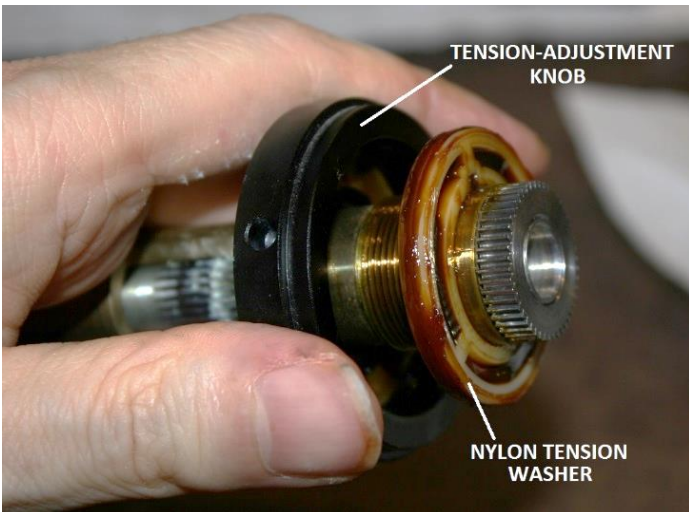
Figure 53 – Remove the nylon tension washer
