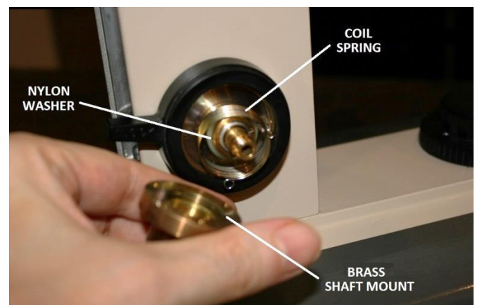
Figure 26 – Spring and nylon washer under shaft mount
