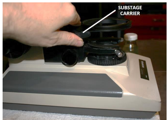
Figure 116 – Lower substage condenser carrier onto rails
