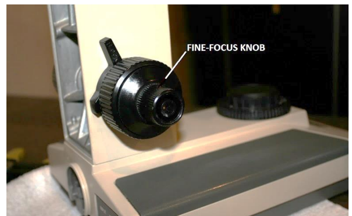
Figure 91 – Reinstall the fine-focus knob (left side shown)
