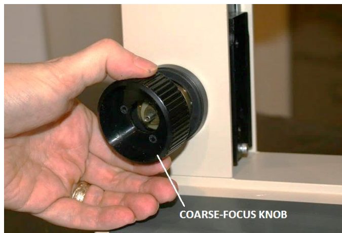
Figure 21 – Remove the coarse-focus knob
