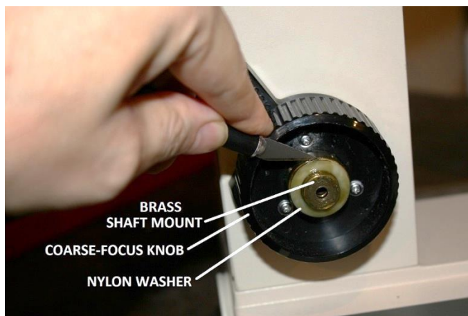
Figure 19 – Remove the nylon thrust washer
