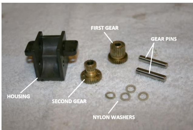
Figure 98 – A view of the gearbox fully disassembled
