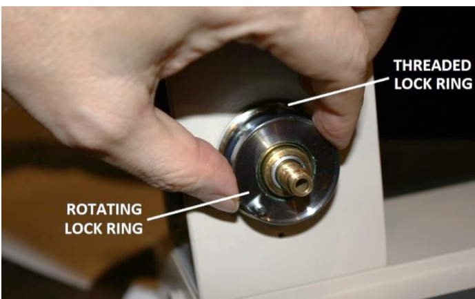
Figure 29 – Remove the rotating lock ring
