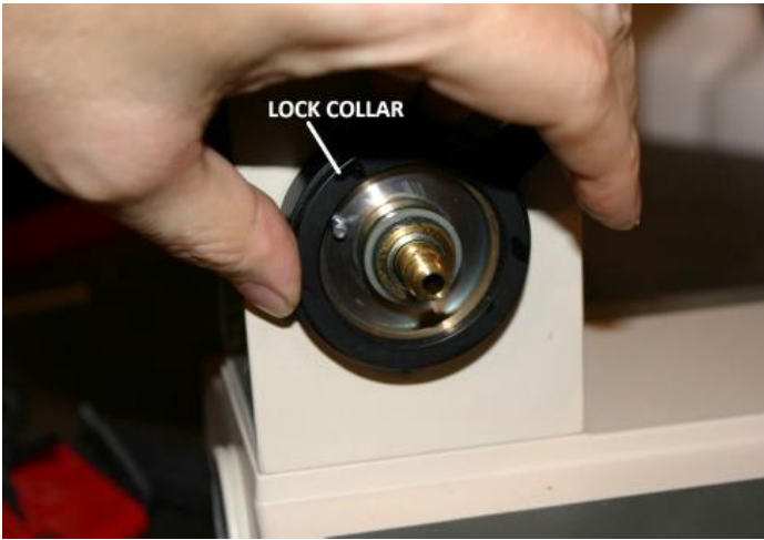
Figure 27 – Loosen and remove the pre-focus lock collar
