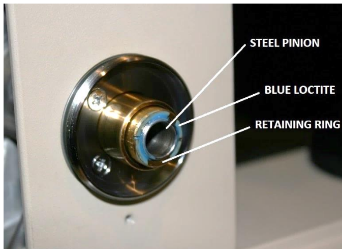
Figure 75 – Apply Loctite® to secure the retaining ring
