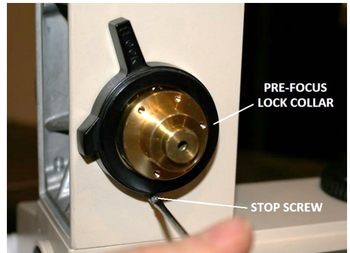
Figure 86 – Reinstall slotted stop screw for lock collar
