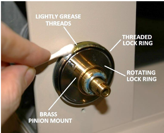
Figure 80 – Lightly grease threads of threaded lock ring
