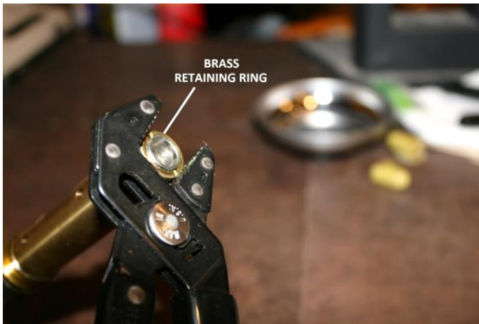
Figure 57 – Loosen and remove the brass retaining ring
