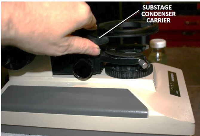
Figure 3 – Lift and remove the substage condenser carrier
