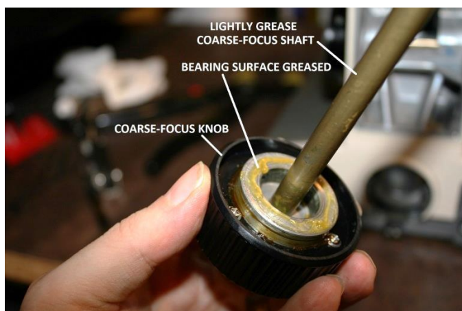
Figure 76 – Apply grease to bearing surface and shaft
