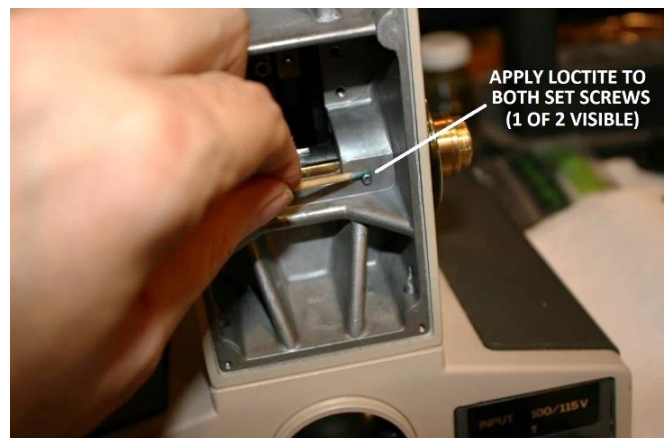
Figure 74 – Apply Loctite® and tighten both set screws
