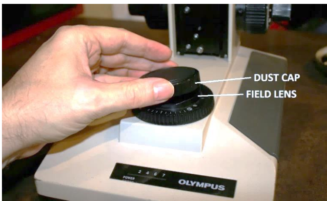
Figure 5 – Protect the field lens with a dust cap
