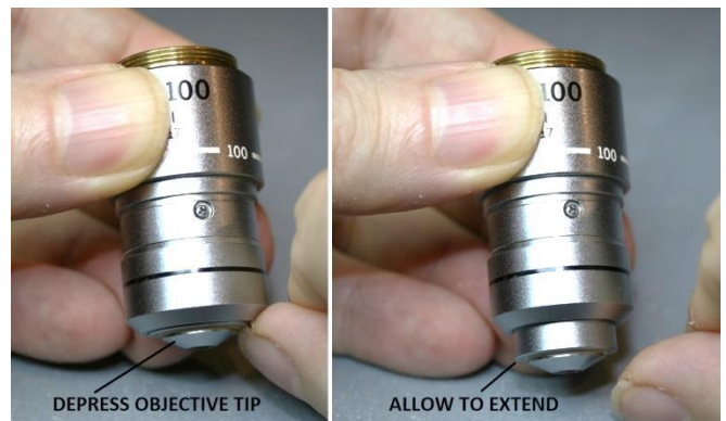
Figure 23 – Test the tip of the reassembled objective
