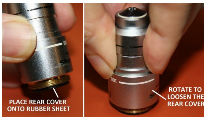
Figure 8 – Loosen the threaded rear cover on rubber sheet
