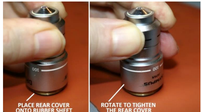
Figure 22 – Tighten threaded rear cover on rubber sheet
