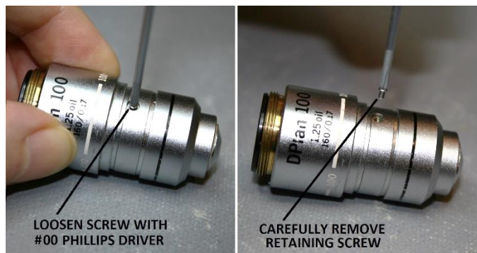
Figure 6 – Remove the small retaining screw
