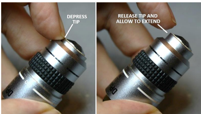
Figure 2 – Test the spring-loaded tip
