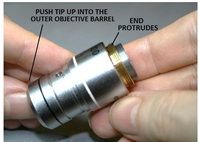
Figure 11 – Push objective tip up into the objective barrel
