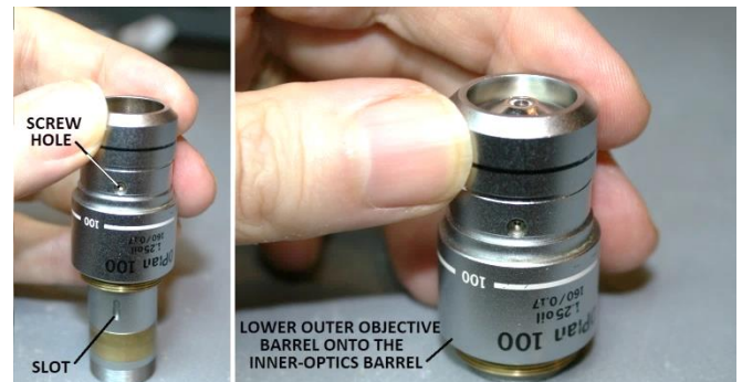
Figure 16 – Place outer barrel over the inner-optics barrel
