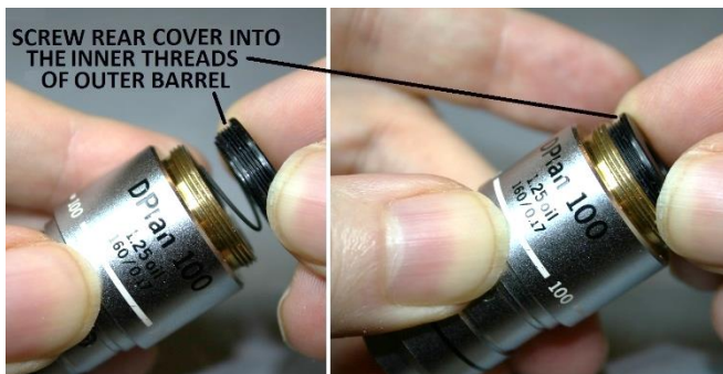
Figure 21 – Reinstall the threaded rear cover
