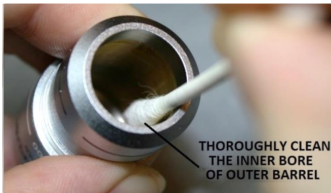
Figure 14 – Clean inner bore of the outer objective barrel
