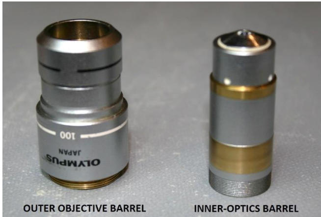
Figure 13 – Inner-optics barrel removed from outer barrel
