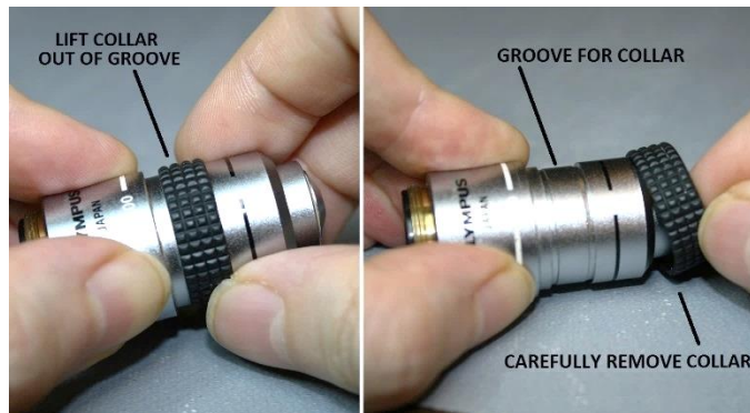
Figure 4 – Remove the knurled-rubber grip collar
