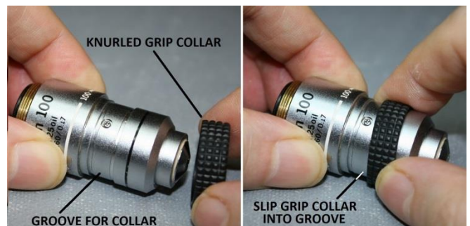
Figure 24 – Reinstall the knurled rubber grip collar
