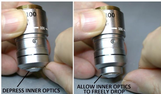
Figure 19 – Depress the tip and allow it to drop
