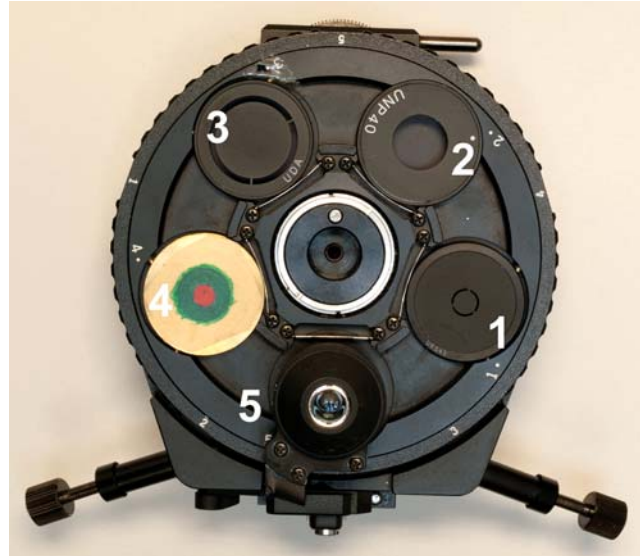
Figure 19. Top view of uncovered Olympus Universal condenser with a five-position turret. Plates in positions are as follows: 1) 40X phase contrast; 2) 40X Nomarski DIC; 3) 40X darkfield; 4) central-red, annular green Rheinberg disc from colored masking tape; and 5) open slot (not observable under top 0.8 N.A. lens).
