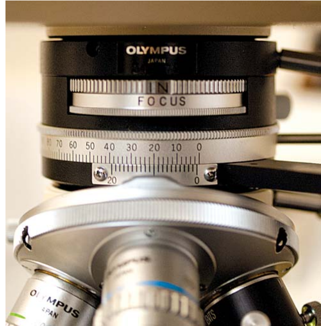
Figure 11. An Olympus Bertrand lens location (focusable) at the "IN" position above the analyzer (graduated) and Red I waveplate. Below the analyzer and waveplate is the turret for the objectives.
