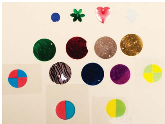
Figure 8. Various stops used for Rheinberg. Four of these — the left-most, right-most and two bottom-most — were printed from a color laser printer. The other discs and the top punched design pieces were gathered from party events.
