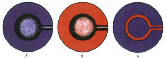
Figure 24. A portion of Plate II from Wright's Principles of Microscopy . Glass beads were viewed with a blue stop, red stop, then blue central and red annular stop. Overlapping adjacent original images have been digitally removed for clarity.
