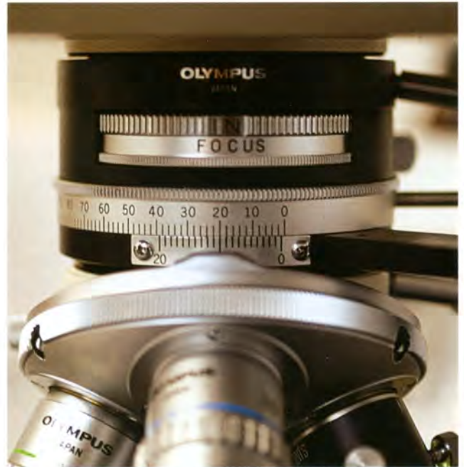
Figure 11. An Olympus Bertrand lens location (focussable) at the "IN" position above the analyzer (graduated) and Red I waveplate. Below the analyzer and waveplate is the turret for the objectives.
