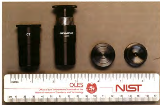
Figure 10. Olympus telescoping lenses (centering telescopes) and pinhole eye caps. From left to right: side view of a telescoping lens, side view of a telescoping lens extended for viewing NBFP or CAFD, a top view of eye cap and a bottom view of the eye cap.
