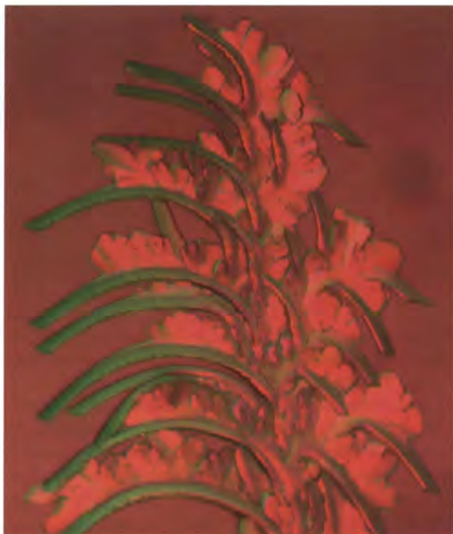
Figure 18. Fusion preparation of the polynuclear aromatic hydrocarbon (PAH) anthracene, often found in fossil fuels. It has a crystal habit of forming scimitar-like blades and lathes; in this case, grouped crystals that look much like a Christmas tree. The central stop portion is red and the outer annulus is green. Actual stop is shown in Figure 19 at insert plate 4.
