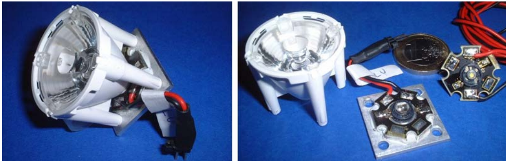
Fig. 1 Pictures representing the LED illuminator. On the left the fully assembled device. On the right the various components: a) the plastic lens condenser, b) the single LED chip and c) the chip mounted on the metal plate.
