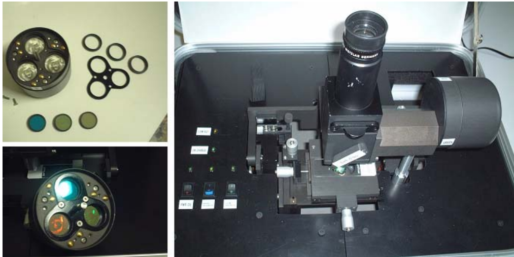
Fig. 4 The portable fluorescence microscope. On the left, details of the rotating multicolor solid state illuminator housing the three LEDs (upper) coupled with the corresponding interference filters (below). On the right the view of the microscope turrette holding the illuminator. The microscope stage with the sample movements as well as the switches controlling bright field and fluorescence excitation can be seen at the bottom.
