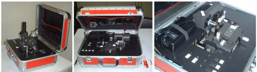
Fig. 5 The portable fluorescence microscope. On the left, the open bag with the microscope “ready-to-use”. In the central picture the microscope is turned in the “close-mode”. On the right the top mobile part of the microscope is placed down to the bottom of the bag. The external 220 vAC can also be recovered inside the bag.
