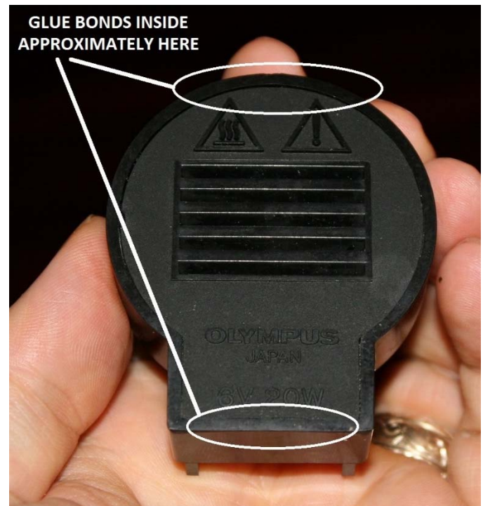
Figure 4 – Locations of adhesive inside the housing
