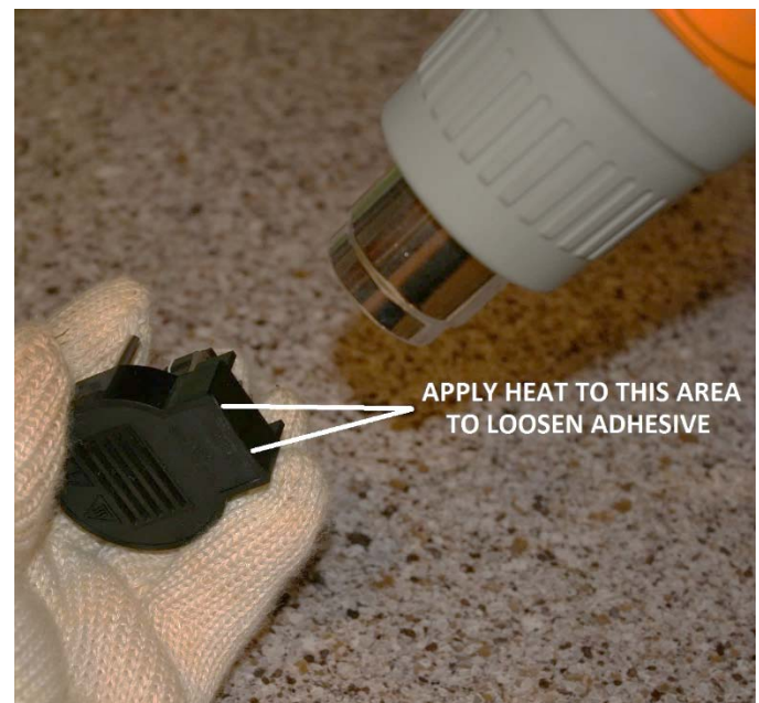
Figure 5 – Apply heat to the flat end to soften the adhesive
