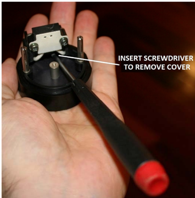
Figure 6 – Use screwdriver to pry the flat end of cover
