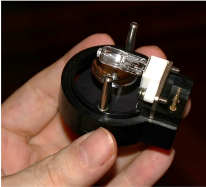
Figure 17 – Refurbished lamp house ready for service
