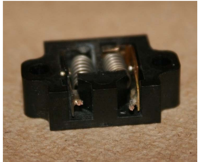
Figure 18 – Cover removed to show oxidized contacts
