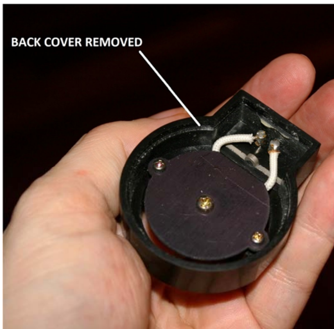
Figure 7 – The lamp house with back cover removed
