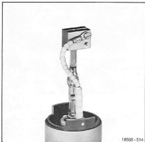
Fig. 21 Lamp inserted in the mount Firmly tighten the screw after insertion of the lamp
