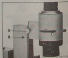
Fig. 16 Inserting the lamp mount 9 Clamping screw of the lamp mount 8 Index 2 for long intercept distance
