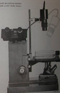
Fig. 29 DIAVERT with special lamp holder for large objects
