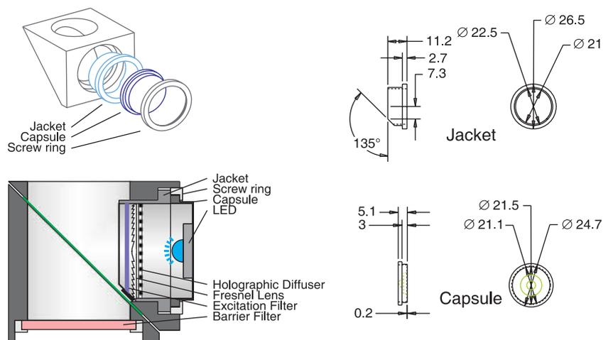
Fig. 1. Schematic drawing of the mountings and filter block. All dimensions in mm. LED, light-emitting diode.
