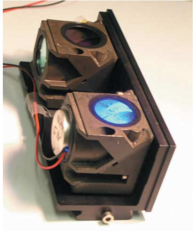
Fig. 2. Photograph of the filter block with capsule and jacket mounted and light-emitting diode switched on.
