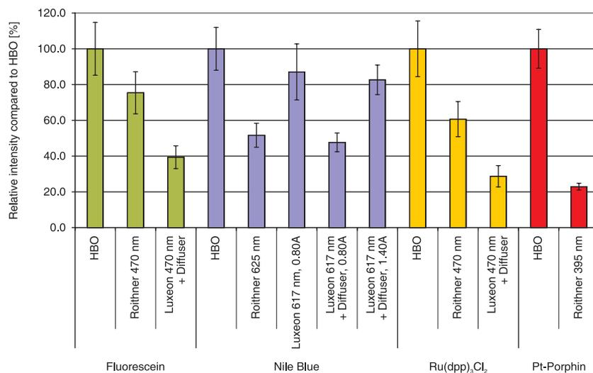
**Fig. 4.** Relative fluorescence intensities obtained for different types of fluorescent microspheres, used as reference specimen. Detailed values and operating conditions are shown in Table 2.
