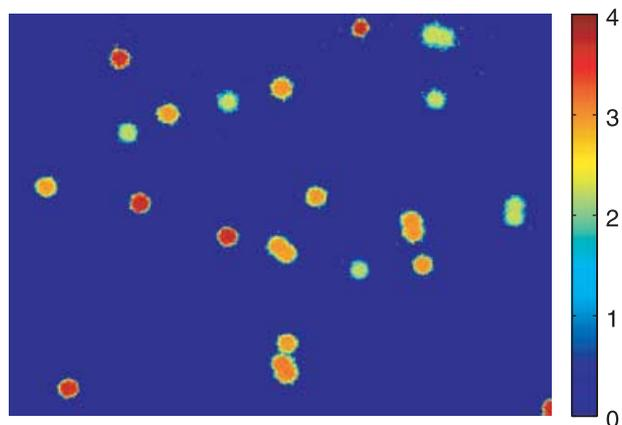
Fig. 5. Fluorescence lifetime image of beads with lifetimes of 3.6, 3.0 and 2.2  $\mu$ s. Field of view is 330  $\times$  250  $\mu$ m.
