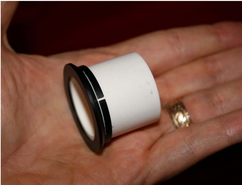
Figure 6: PVC pipe section snapped into Nikon MXA20495 filter holder
