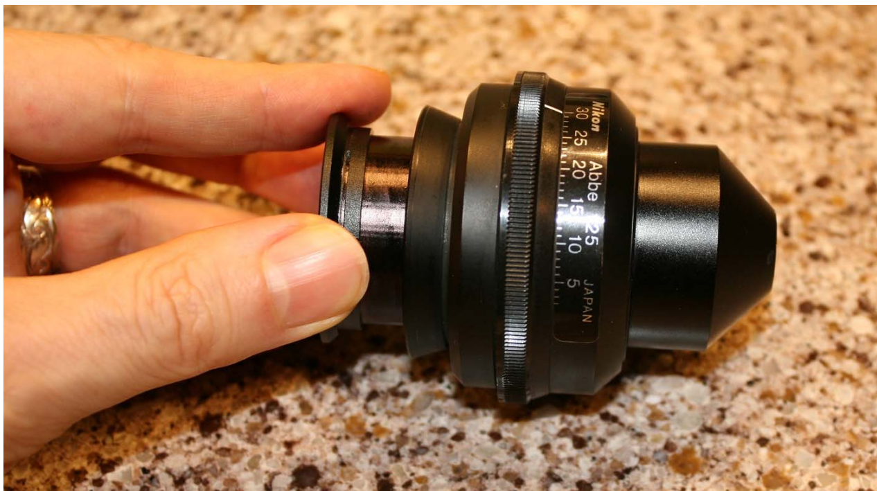
Figure 10: Installing the finished darkfield insert into the Nikon condenser
