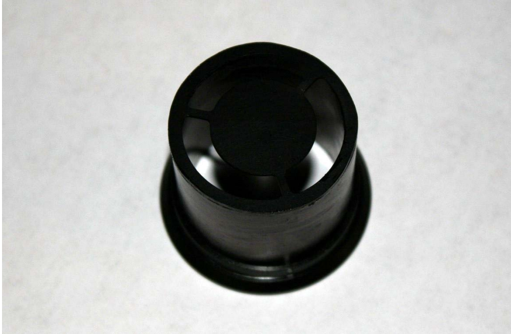
Figure 9: The finished darkfield insert, after “blacking” the pipe and assembling the pieces
