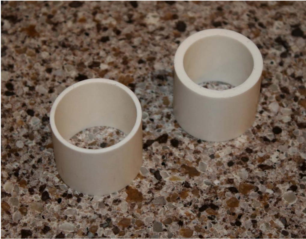
Figure 5: A view of the difference in wall thicknesses in SDR-21 PVC (left) and Schedule 40 PVC (right)
