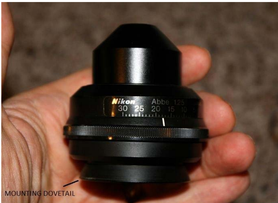
Figure 1: Abbe condenser from Nikon Labophot
