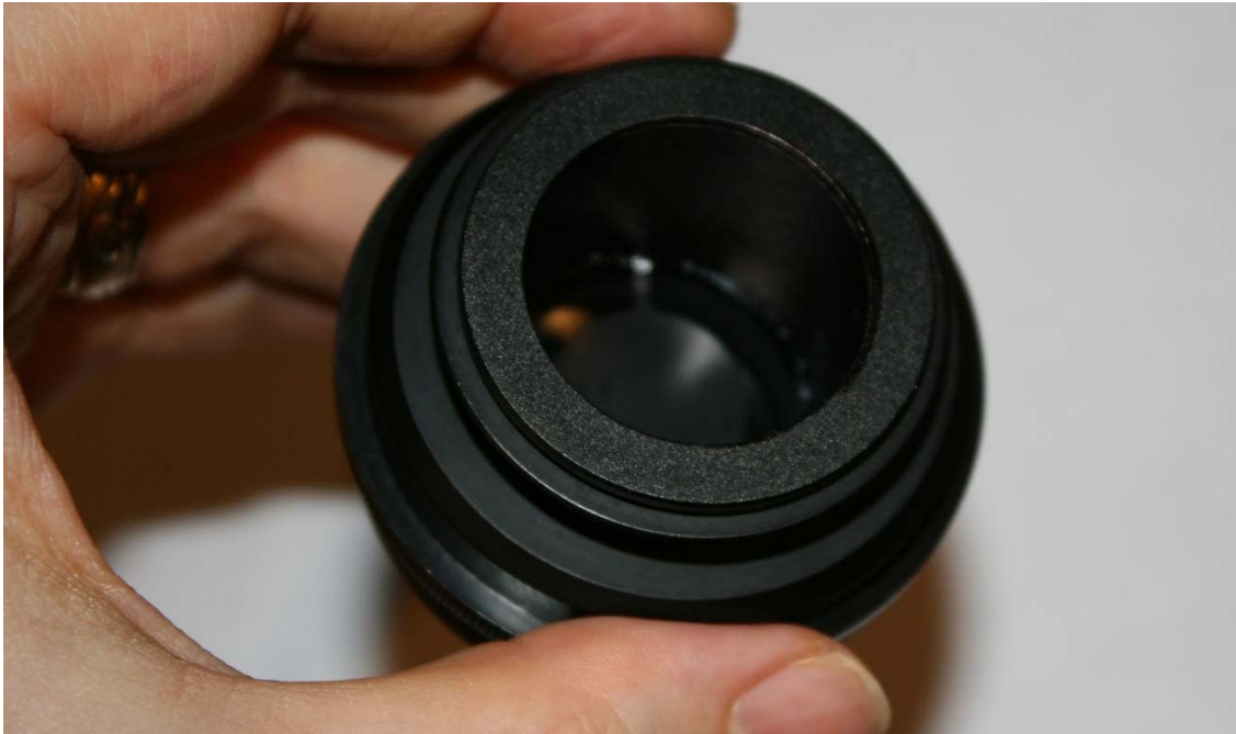
Figure 11: The Nikon condenser equipped for darkfield
