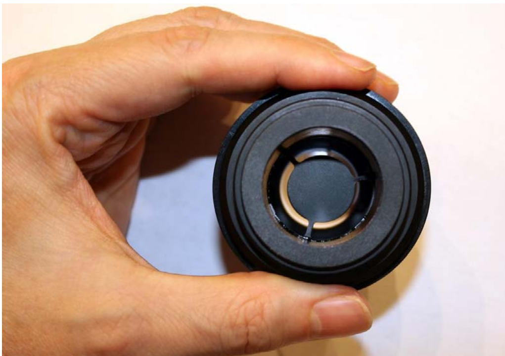
Figure 12: Looking into the under-bore of the darkfield-equipped Nikon condenser
