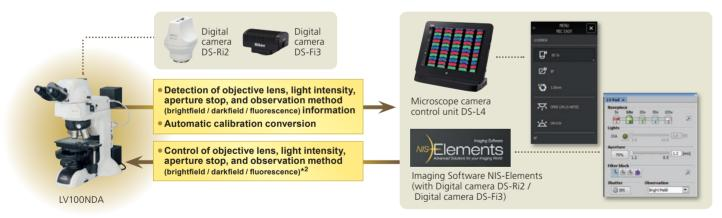
\*2: Information detection only, when the control unit DS-L4 is connected. Control of the objective lens, light intensity, aperture stop, and observation method (brightfield / darkfield / fluorescence) is possible when the DS-Ri2 or DS-Fi3 (with NIS-Elements) is connected.
