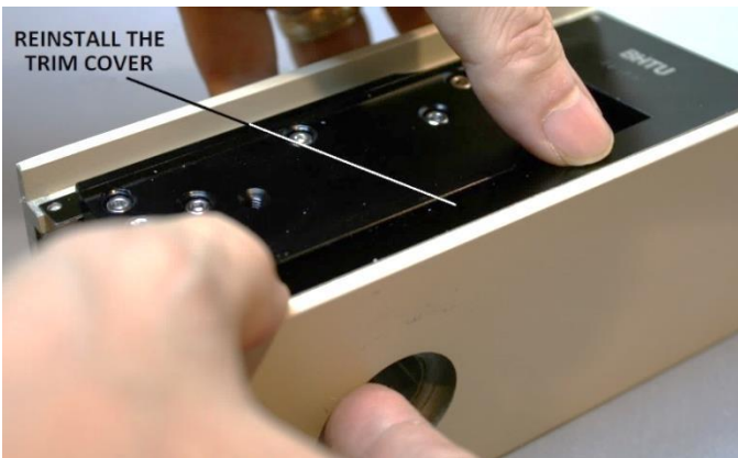
Figure 51 – Reposition the trim cover onto the arm
