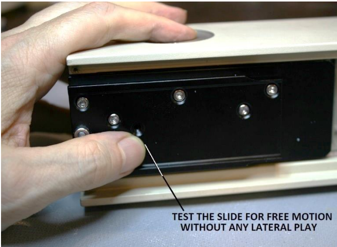
Figure 50 – Test the sliding focus block for proper motion
