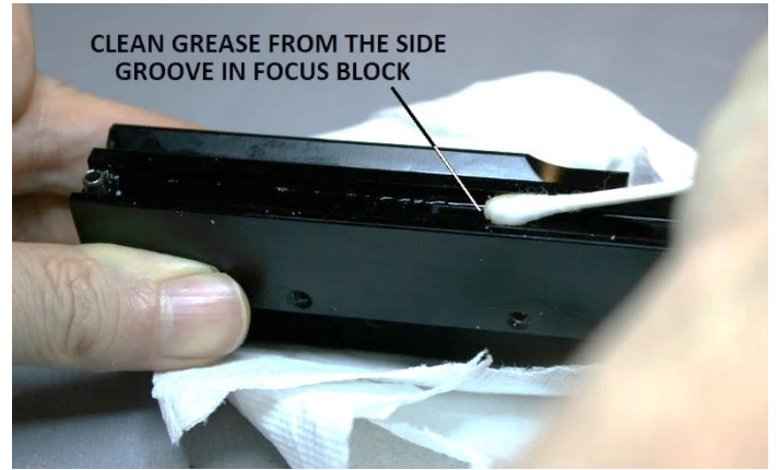
Figure 22 – Clean grease from side groove in focus block
