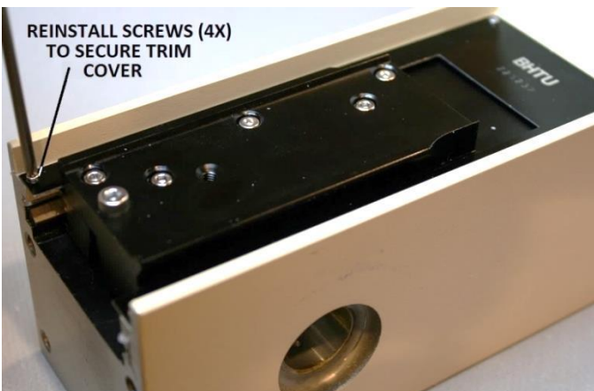
Figure 52 – Reinstall screws to secure the trim cover
