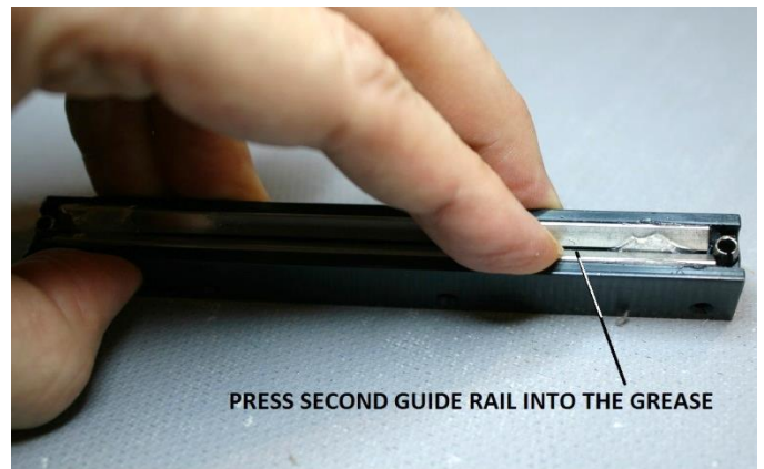
Figure 66 – Set the second guide rail into the grease
