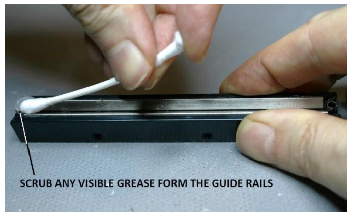
Figure 67 – Scrub any visible grease from the guide rails
