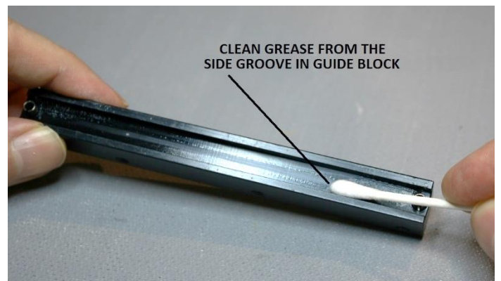
Figure 24 – Clean grease from side groove in guide block
