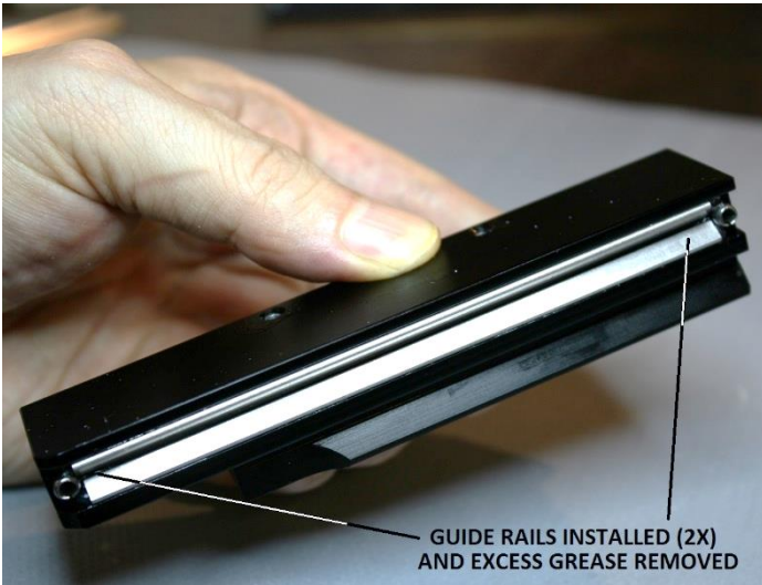
Figure 31 – Guide rails installed into the focus block
