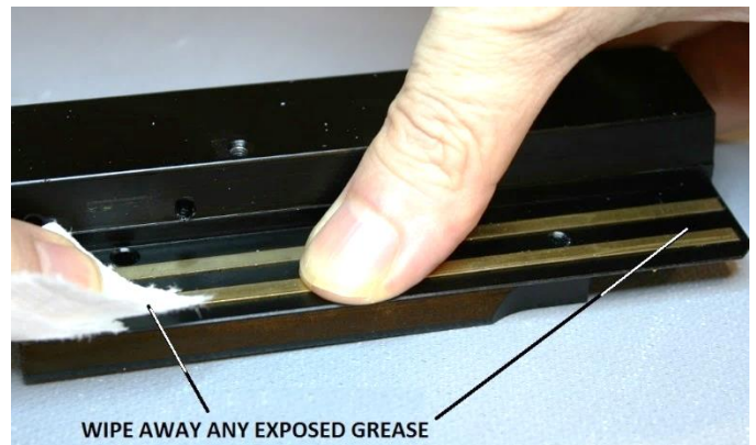
Figure 36 – Clean exposed grease from the focus block
