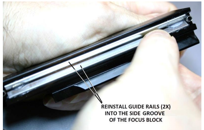
Figure 29 – Reinstall short guide rails into the focus block
