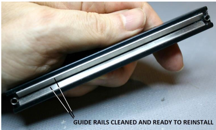
Figure 68 – Cleaned guide block is ready for reinstallation
