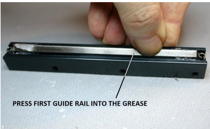
Figure 64 – Set the first guide rail into the grease
