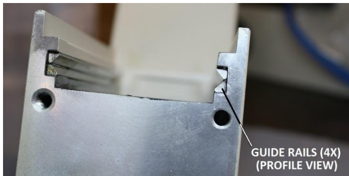
Figure 59 – Correct orientation of the guide rails
