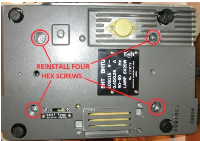
Figure 57 – Reinstall screws to secure the electrical base
