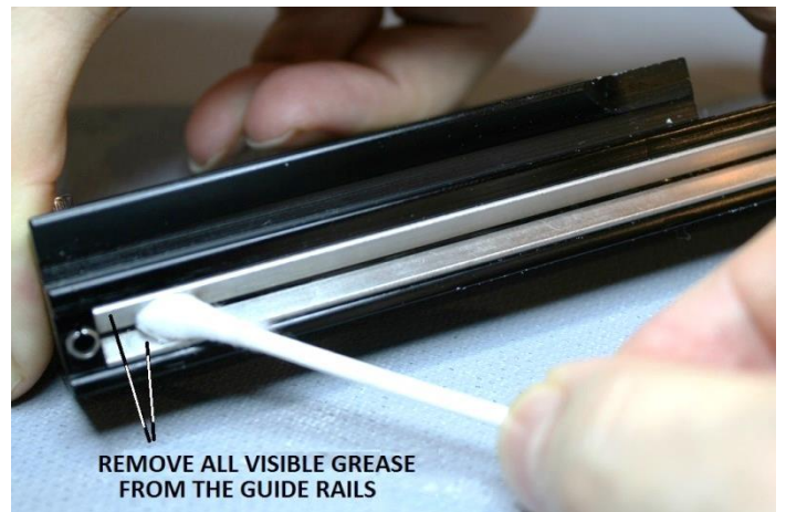
Figure 30 – Scrub grease from guide rails and focus block
