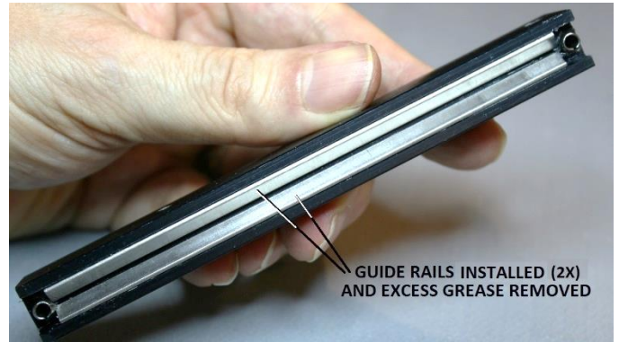
Figure 34 – Guide rails installed into the guide block
