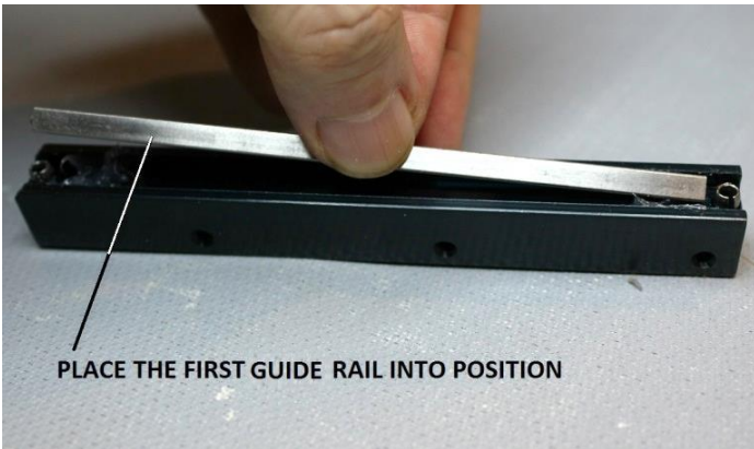
Figure 63 – Place first guide rail into the guide block
