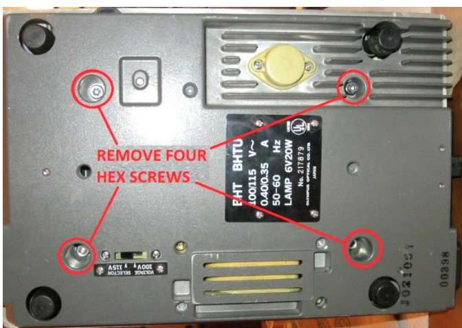
Figure 4 – Bottom view of the BHT/BHTU electrical base
