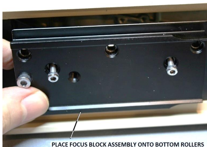
Figure 40 – Place focus block assembly onto rollers
