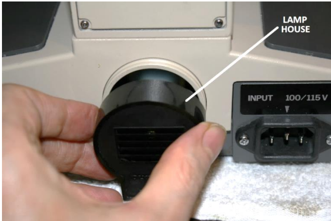
Figure 3 – Remove the lamphouse from the base
