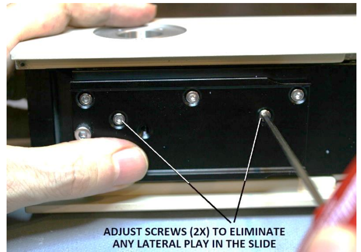
Figure 48 – Adjust for free motion without lateral play
