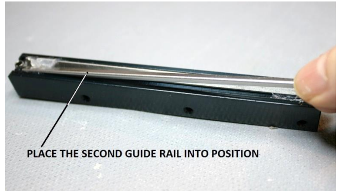
Figure 65 – Place second guide rail into the guide block
