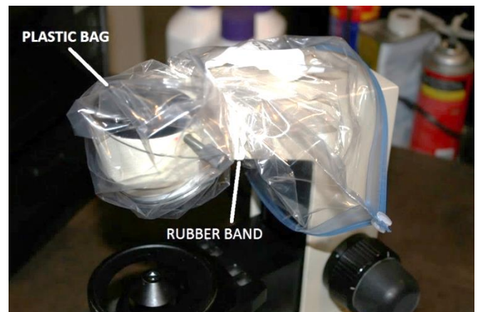
Figure 2 – Protect the top of the arm from dust
