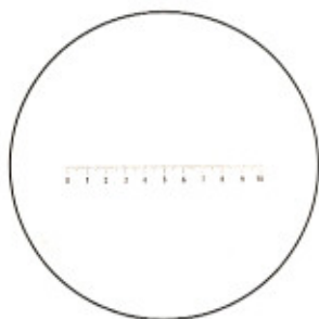
Fig. 4.1 Standard measuring graticule. 1 cm ÷ 100 (M047312).
