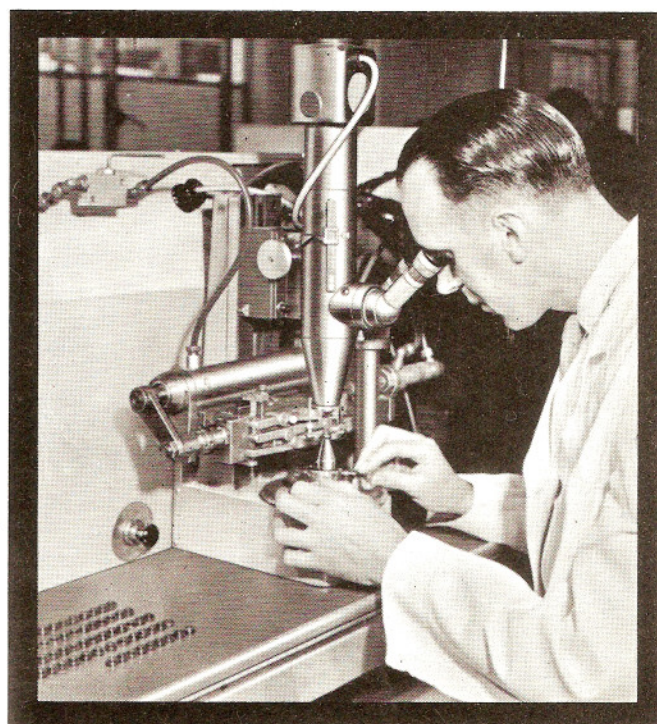
Lens cells for objectives are centred and turned on special purpose high precision machines designed by ourselves.
