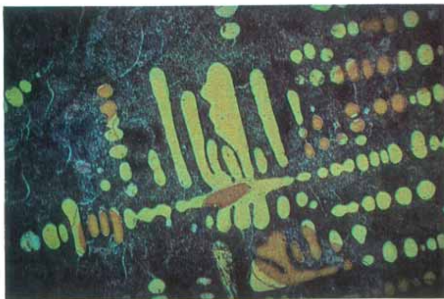
Modified sandcast aluminium alloy Franchini etch—Microplan 10X
