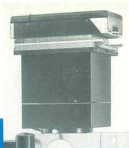
Large format camera assembly with Polaroid CB.100 back
