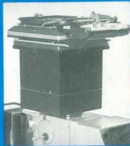
Large format camera assembly with Polaroid 800 back
