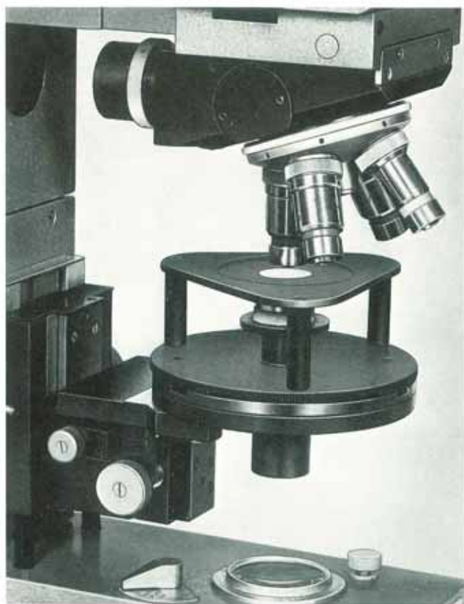
Autolevelling gliding stage
