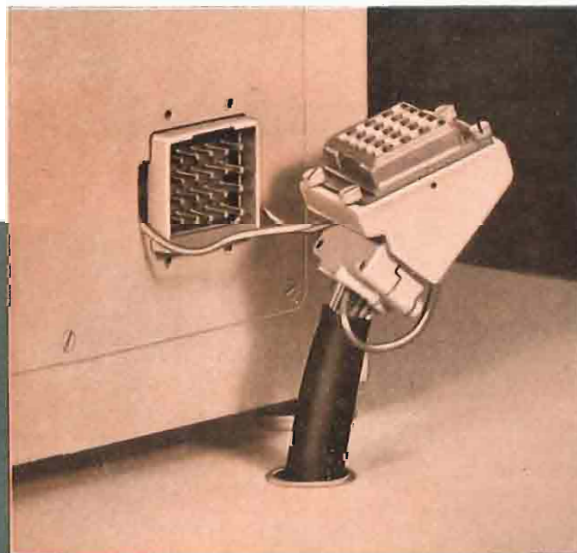
20-way plug connecting the instrument to the built-in power supply unit.
