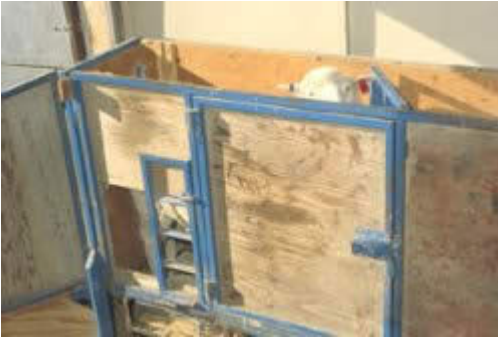
In a just-completed 2-year study, researchers put the hind legs of aging ewes—a model for osteoporosis in people—on this vibrating platform for a daily shake. The vibrated legs lost less bone than the animals' untreated forelegs. Depending on the frequency of the vibrations, some bones gained mass. Simon Turner, Colorado State University
