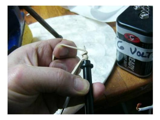
20. Apply tape over the rubber band and the end of the probe to keep it tightly together and to cover all bare metal.
