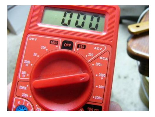
16. Here is another meter that is different colour but does exactly the same thing, shown set to 2 milliamps, or 2000 microamps on the other meter. This is saying the same thing, but with less zeros. Set it here when using godzilla, turn it OFF when done.
