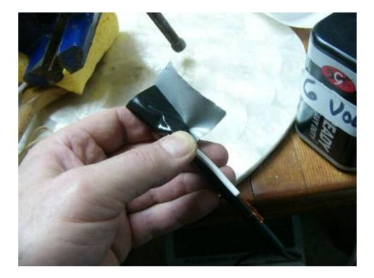
22. Connection between wire and end of probe is now taped and under the tape is the rubber band to hold it very tight. If you just used tape it might work loose.
