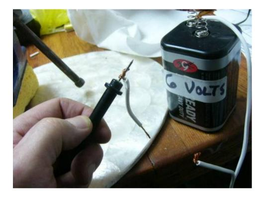
19. First wrap the wire, and then wrap a rubber band tightly over it to get good contact between the wire and the probe. The wire is hidden under the rubber band in the photo.
