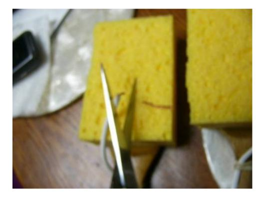
32. Before cutting wires shorter, try rinsing sponges several times in warm water, and squeezing out thoroughly. If still too much power, try reducing power by cutting wires shorter. If still too hot, cut another slit in sponge closer to the wood handle and put wire into it. This will add more sponge between wire and skin.
