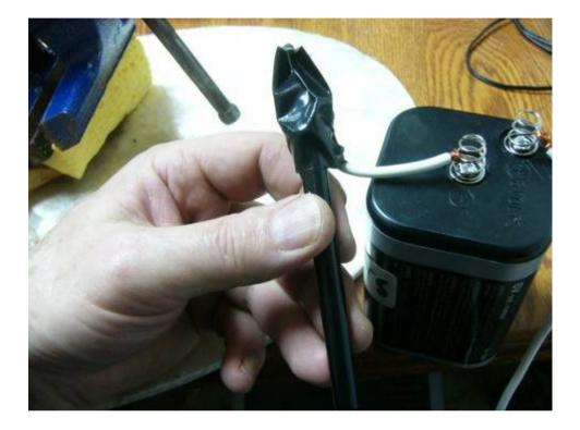
24. Do the same thing with the other probe, attach the wire firsts, then apply rubber band.
