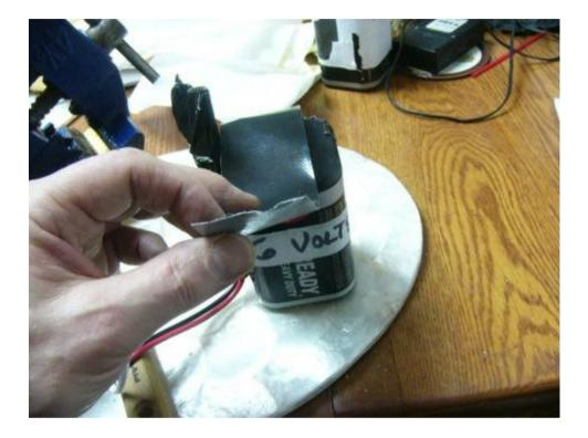
29. Wrap rubber band, tape or zip tie, etc to keep wire inside of sponge to avoid electrical sparks or loss of battery power. You can remove the wires for washing the sponges. You should not have to wash them more than once a year or so, they do not have to be very clean in order to work, and electricity will kill the germs anyway.
