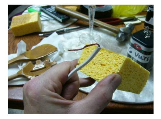
3. Insert bent wire into slit so it reaches into middle of sponge and bare wire is deep inside.
