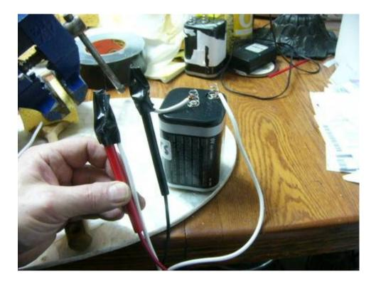
27. Place the two probes upright, along with the wires and tape it all to the side of the battery so the battery can stand up.
