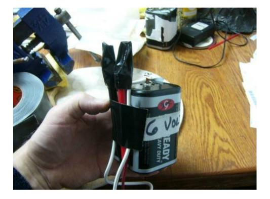
28. Tape over the top. Be sure to cover the metal connections on top of the battery with tape so they do not work loose, and do not touch things to cause sparks or lose the battery charge.
