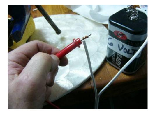
18. Wrap the short bit of wire around the other probe, in this case the black one.
